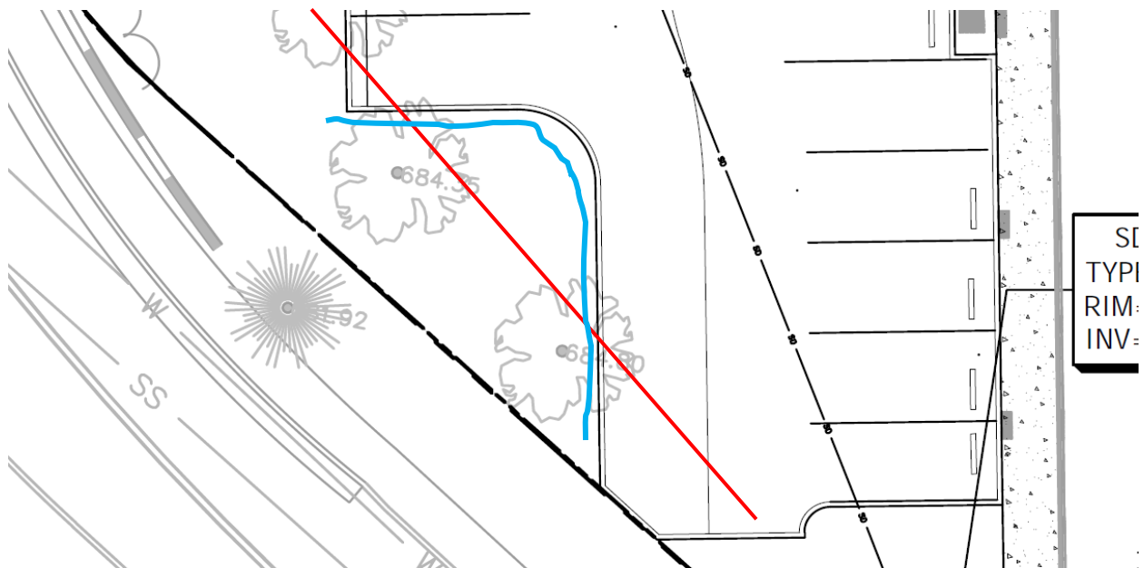
Image #9 – Trees T11 & T12, liquidambar. Note new curb installed adjacent to trees. Some of the new curb will be installed in the same footprint as the existing parking lot (red line is existing curb location). Existing roots will be cut behind new curb (blue line).
