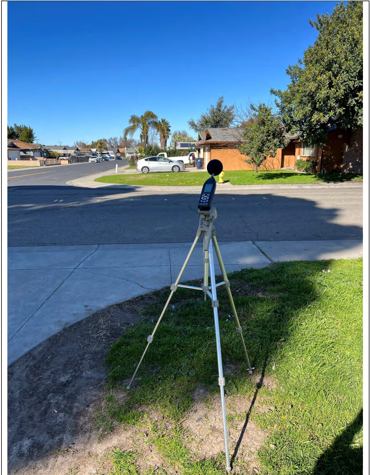
Noise Measurement Survey
