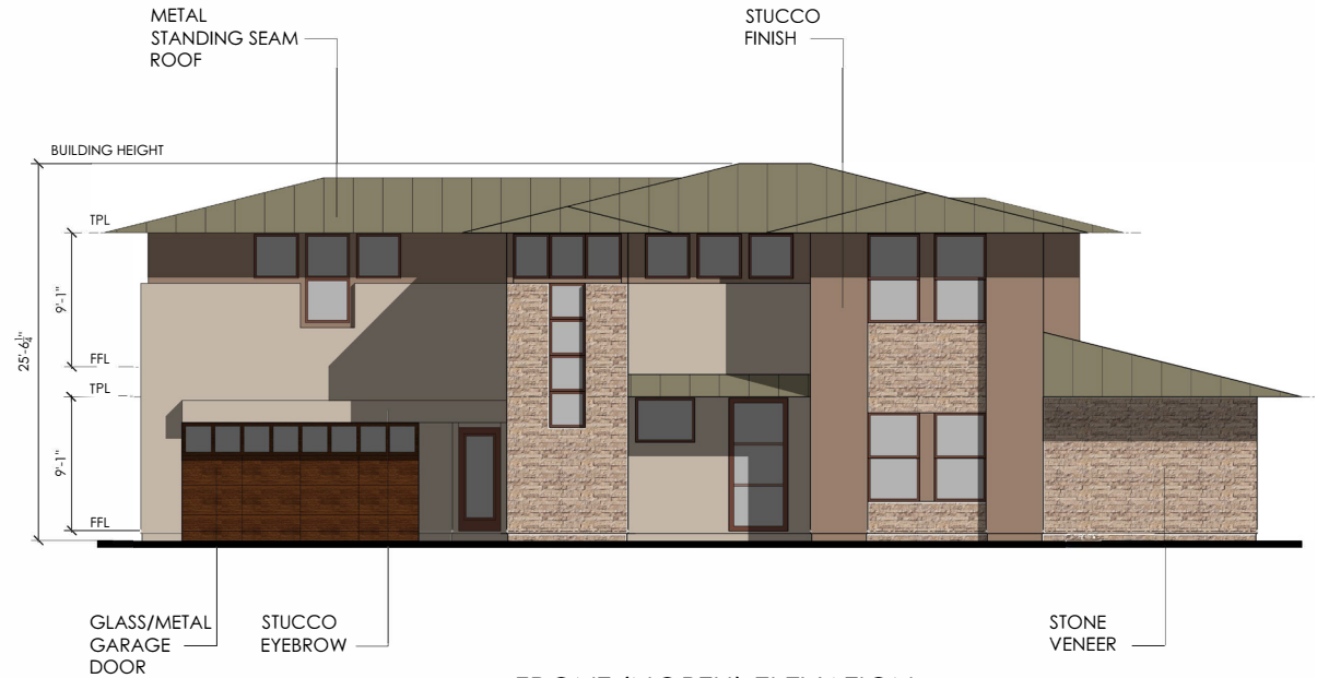
FRONT (NORTH) ELEVATION
