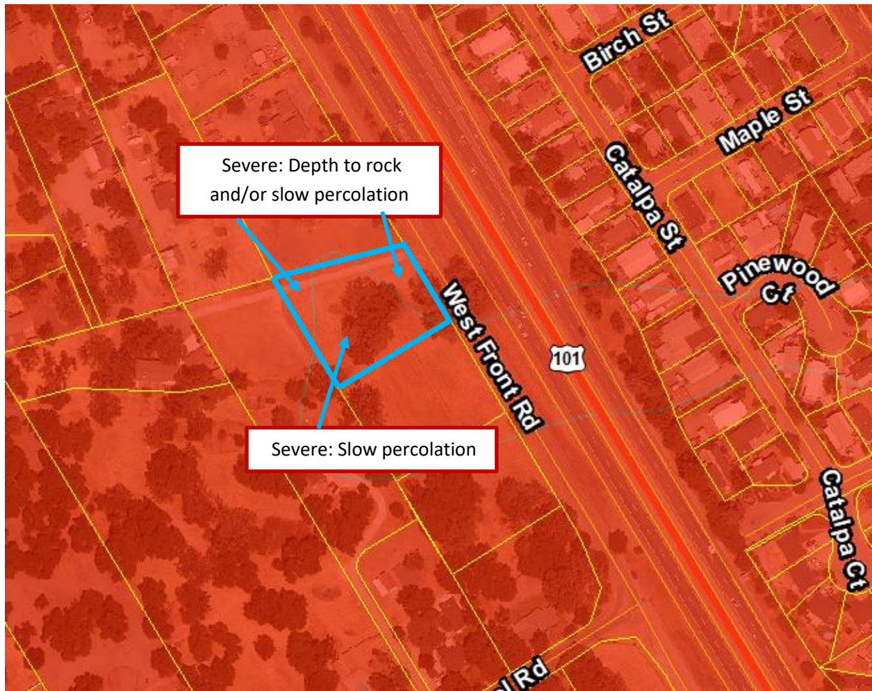
Figure 9 – Soil Septic Suitability
