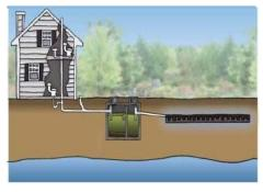
The septic tank is a concrete, fiberglass, Polyethylene or steel box about nine feet long and five feet deep and wide. The tank is usually buried about five feet from the house under one to three feet of soil. The leachline is a gravel-filled underground
