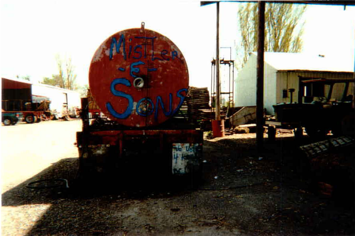
Photograph No. 9. View of diesel tanker trailer (AST) in center of Mistler property looking east. Tanker is currently being used to provide diesel fuel to the farm equipment. Notice large stain in soil behind trailer.
