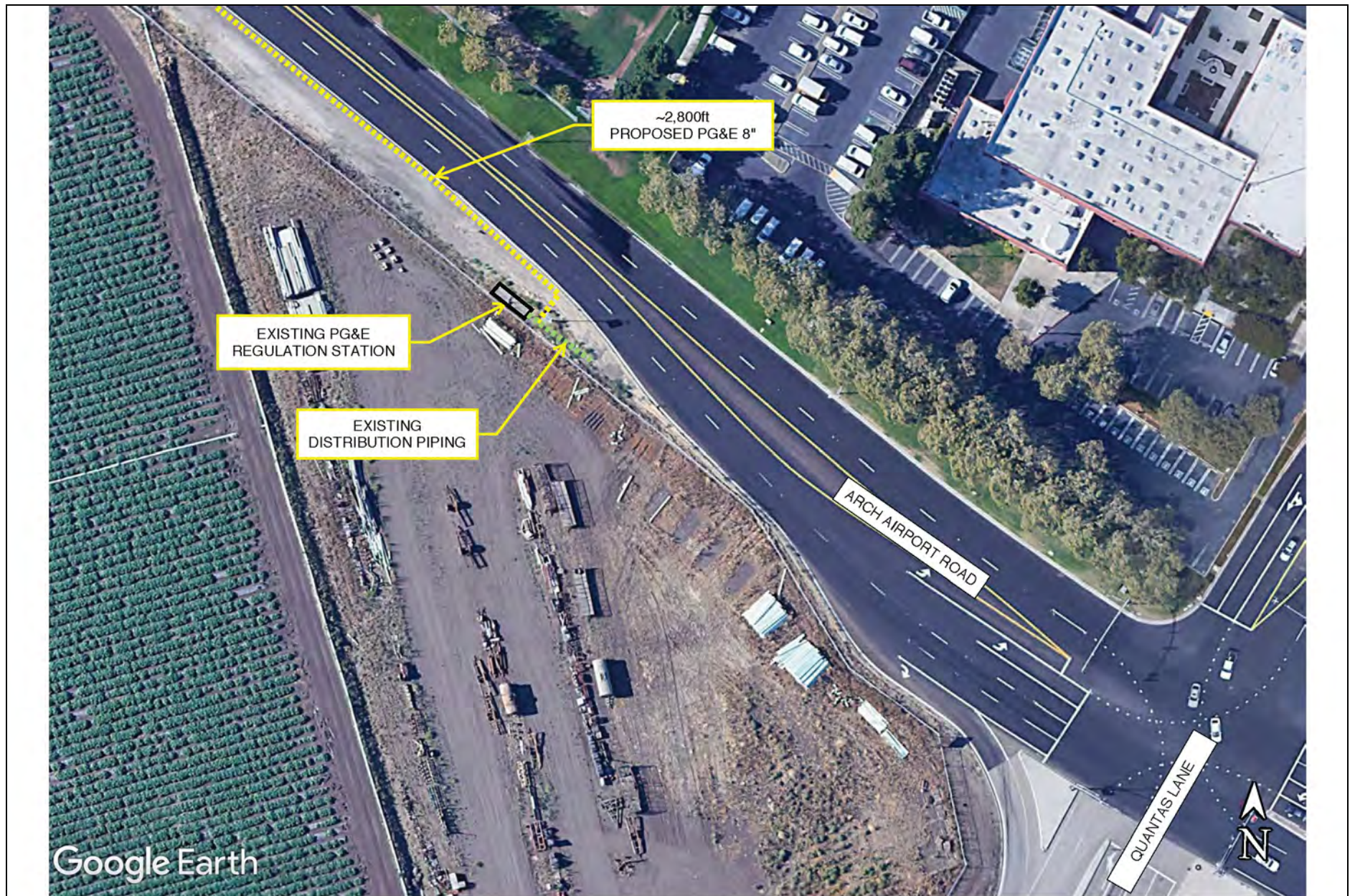
Figure 8 PG&E Regulation Plant and Associated Pipelines
