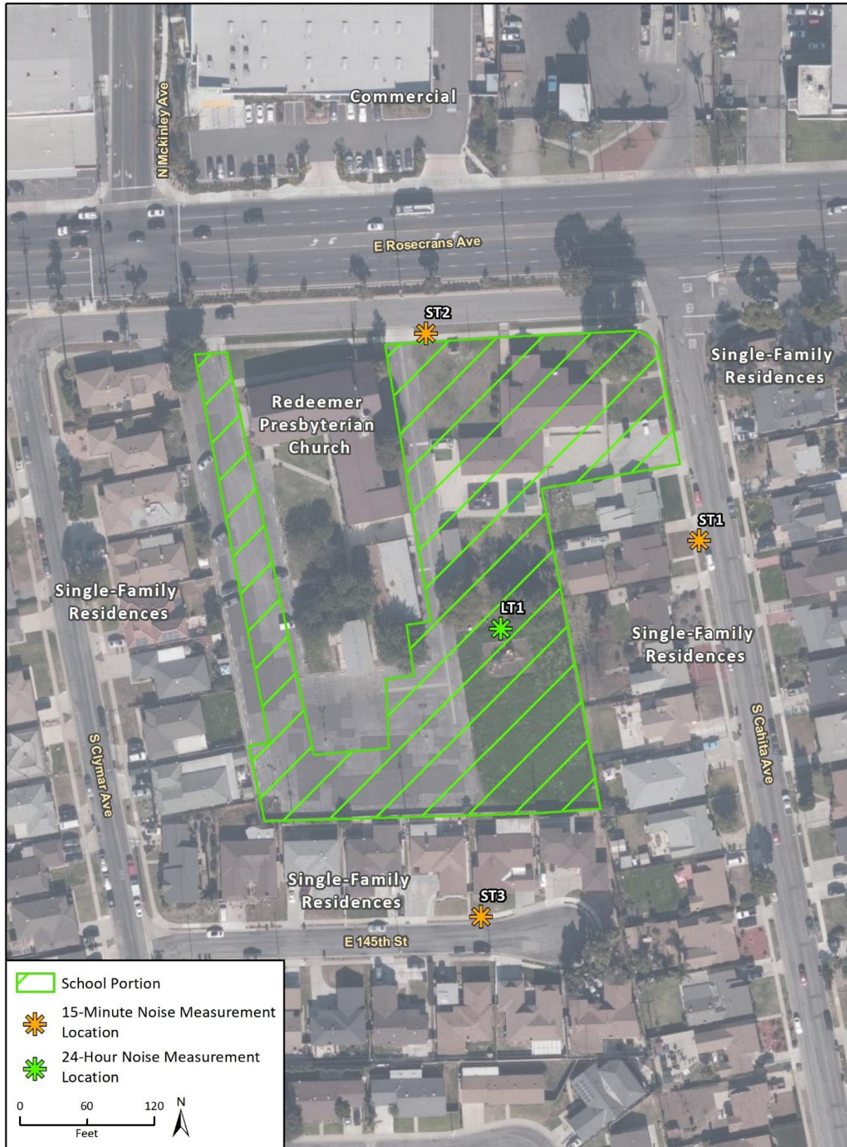
Figure 4 Noise Measurement and Sensitive Receiver Locations
