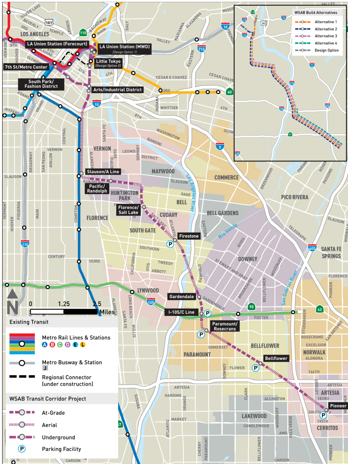
Figure 2-4. Project Alignment by Alignment Type
