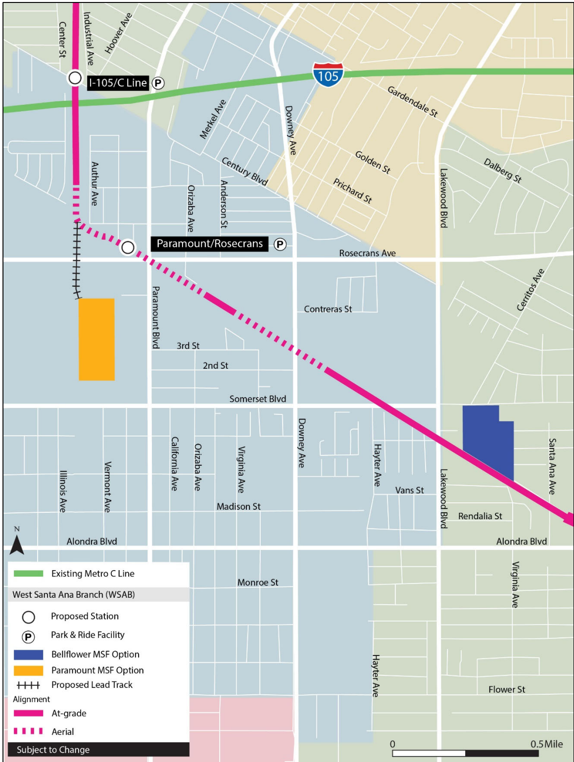
Figure 2-7. Maintenance and Storage Facility Options
