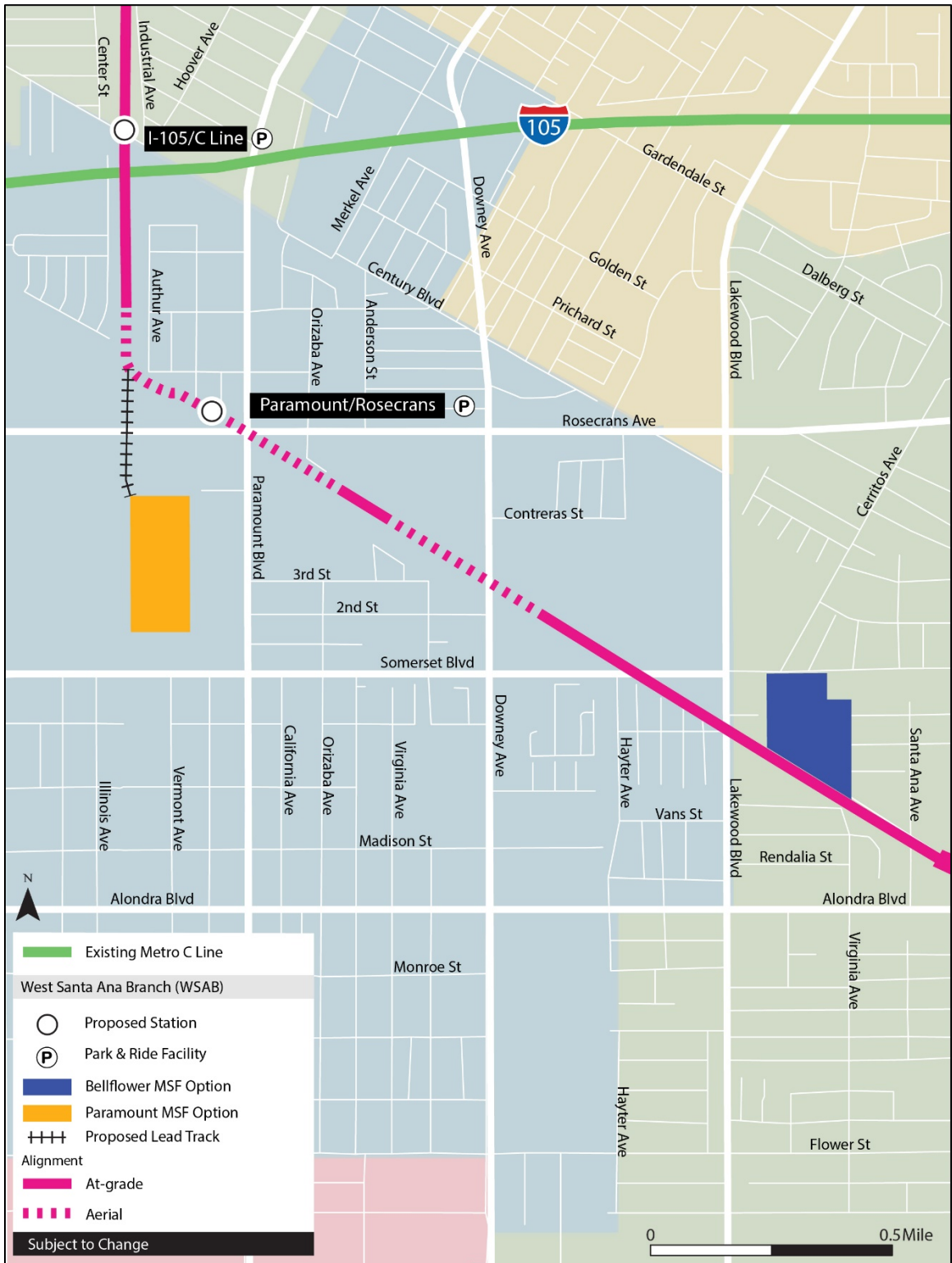
Figure 2-7. Maintenance and Storage Facility Options
