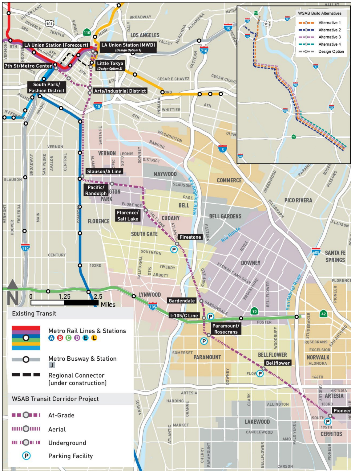
Figure 2-2. Project Alignment by Grade
