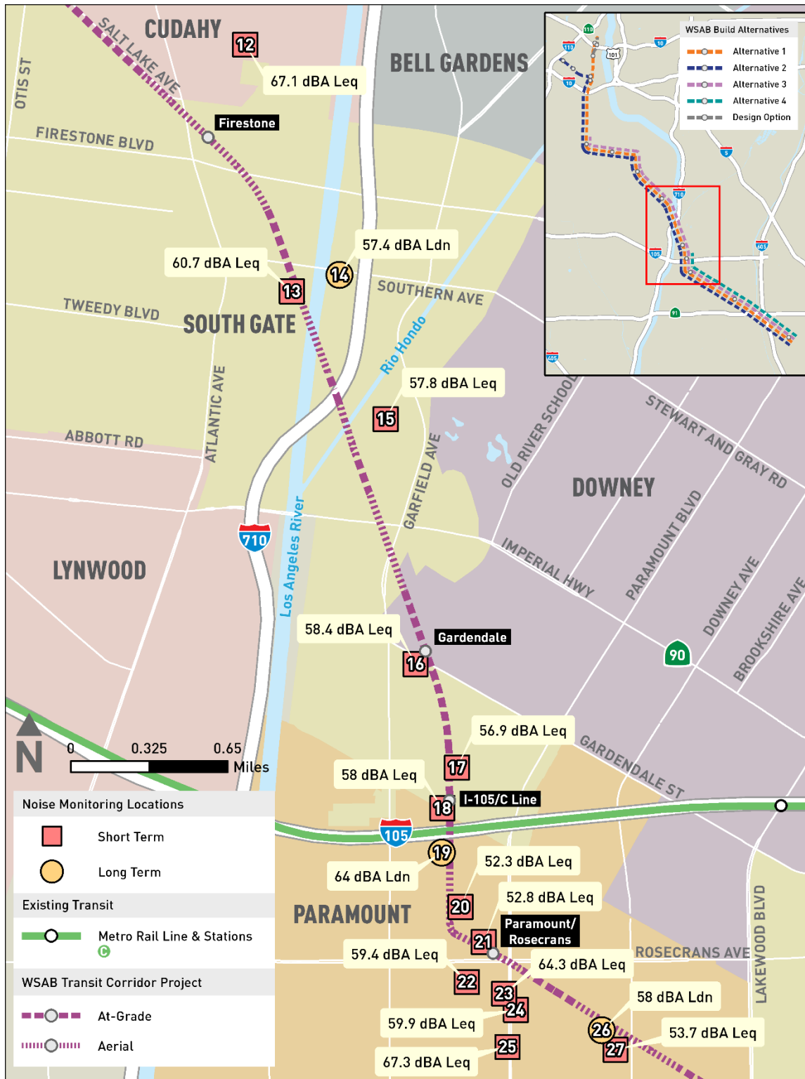
Figure 4.7-3. Noise Monitoring Locations and Existing Noise Levels
