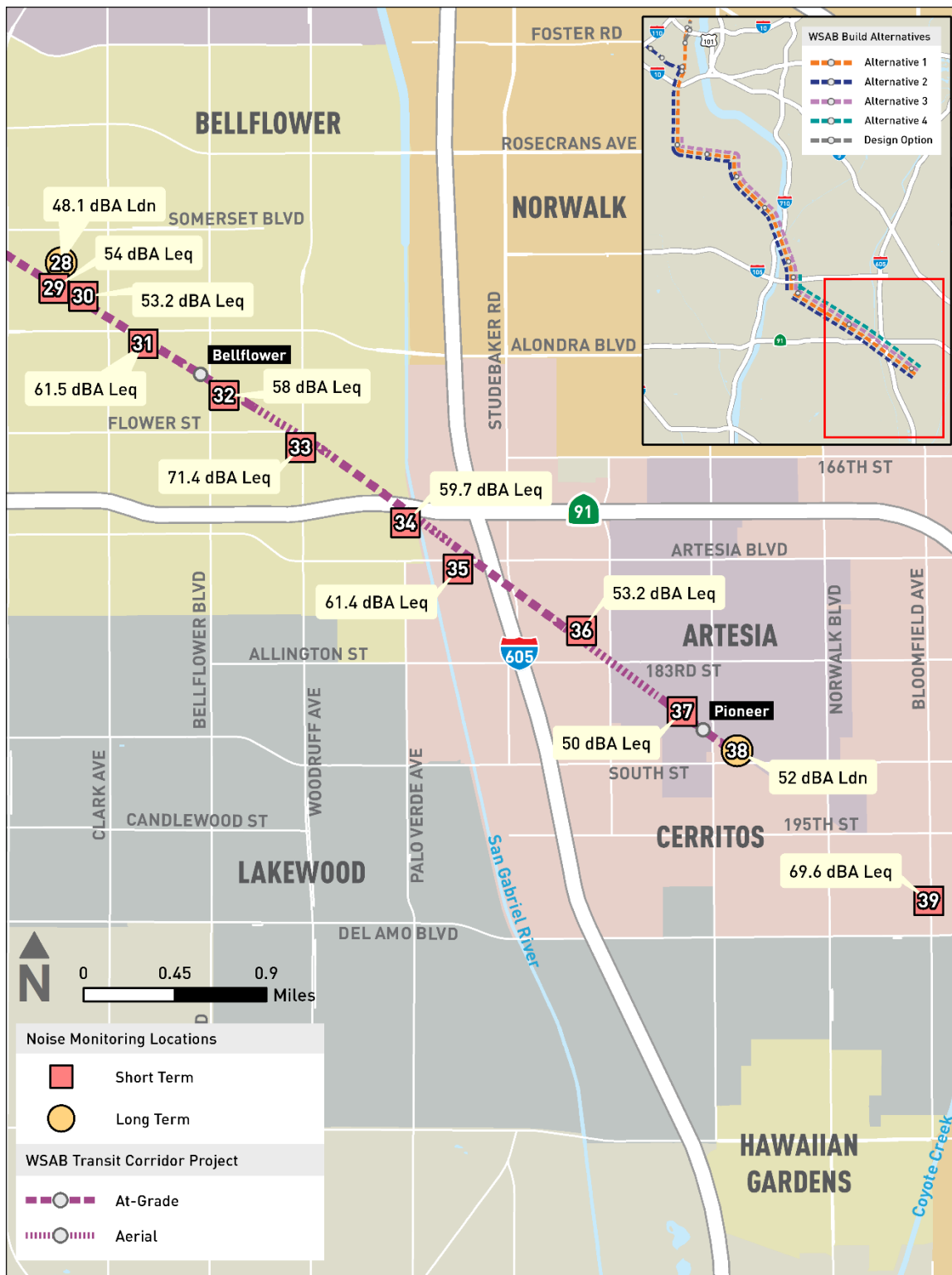
Figure 4.7-4. Noise Monitoring Locations and Existing Noise Levels
