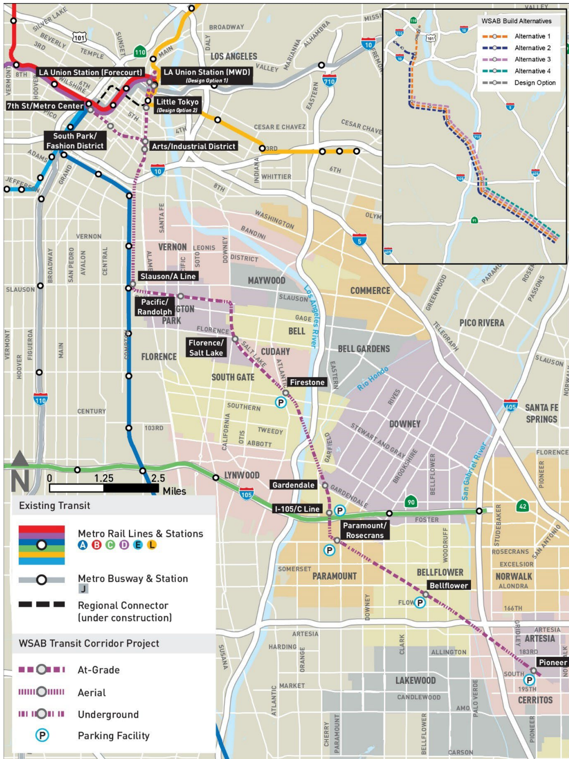
Figure 2-2. Project Alignment by Alignment Type
