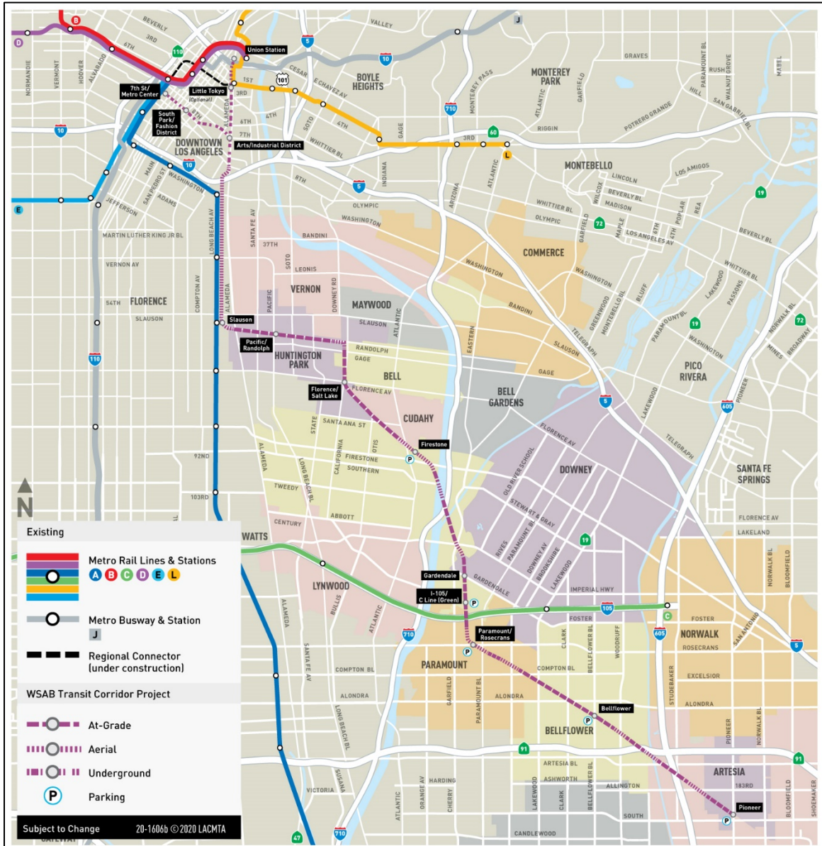
Figure 2-2. Project Alignment by Grade
