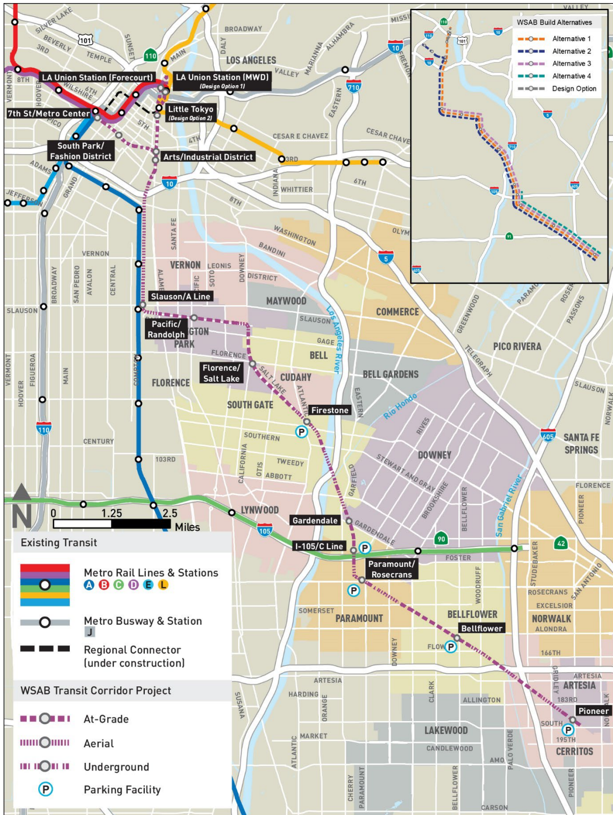
Figure 2-2. Project Alignment by Alignment Type
