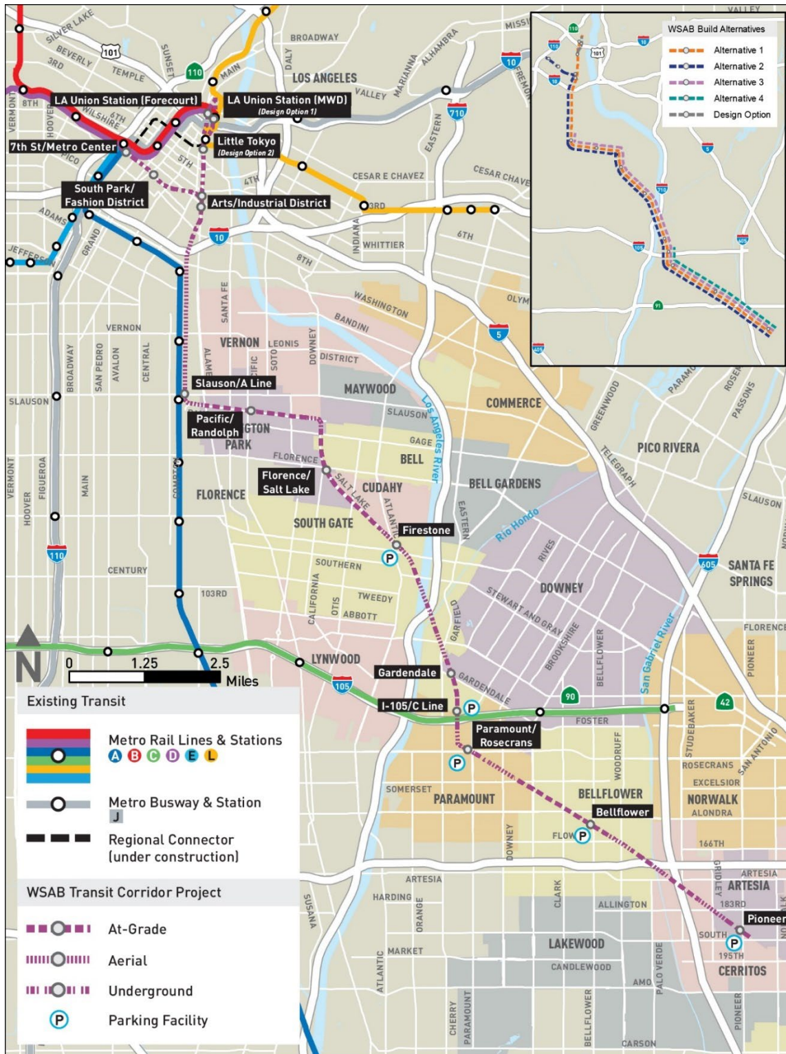
Figure 2-2. Project Alignment by Alignment Type
