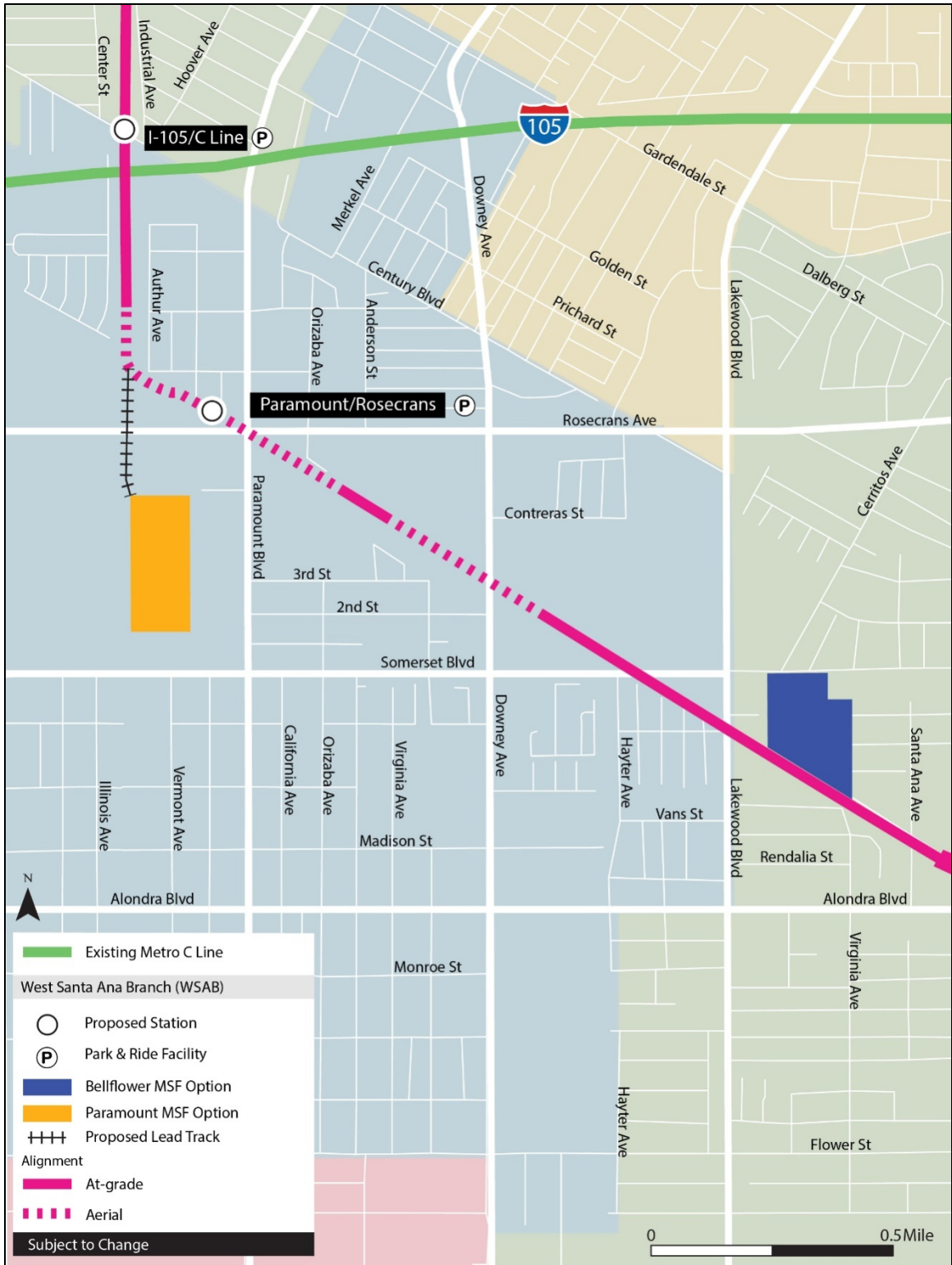
Figure 2-7. Maintenance and Storage Facility Options
