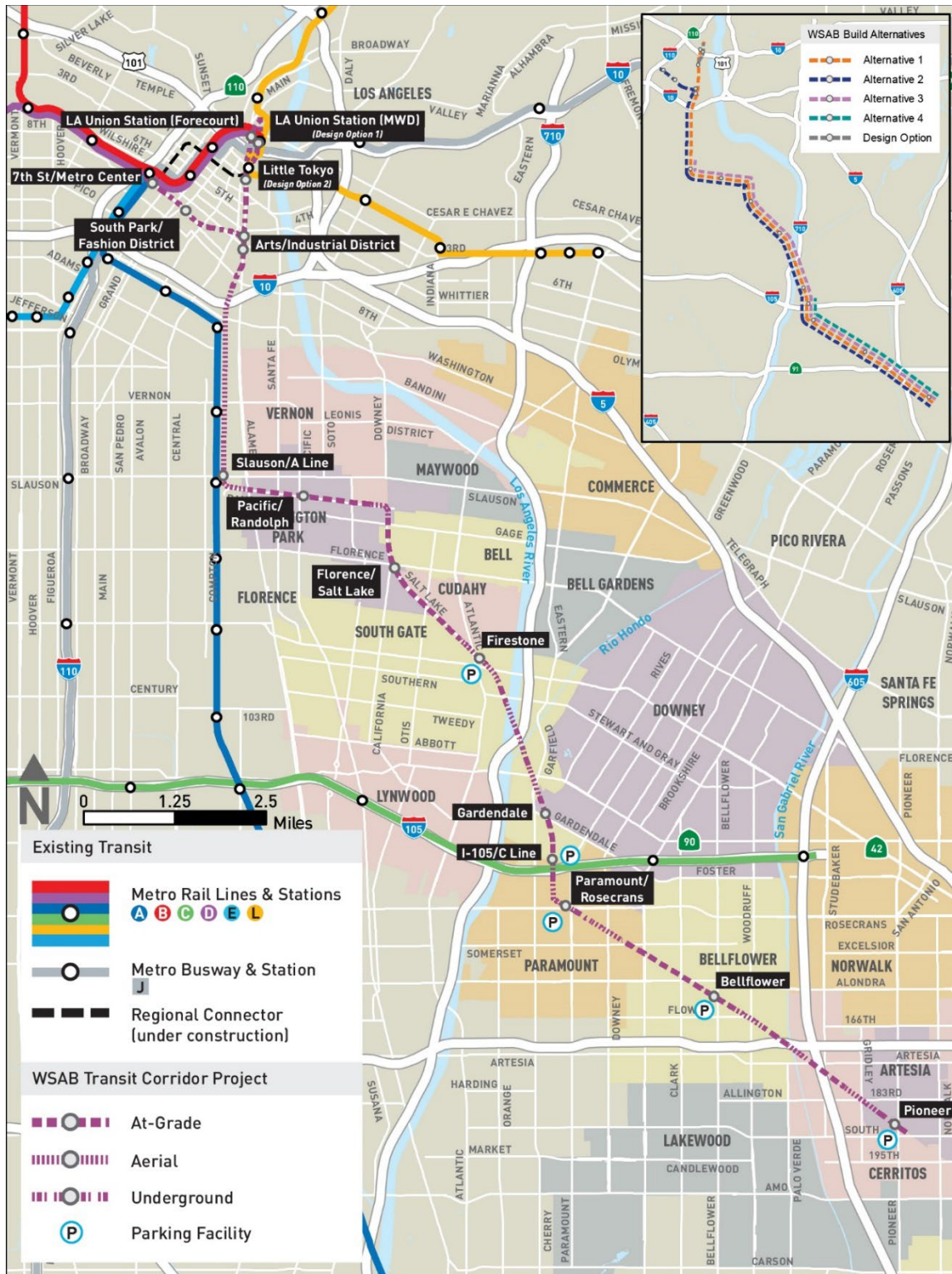
Figure 2-2. Project Alignment by Alignment Type
