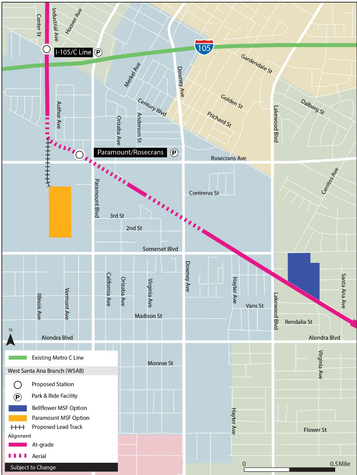
Figure 2-7. Maintenance and Storage Facility Options
