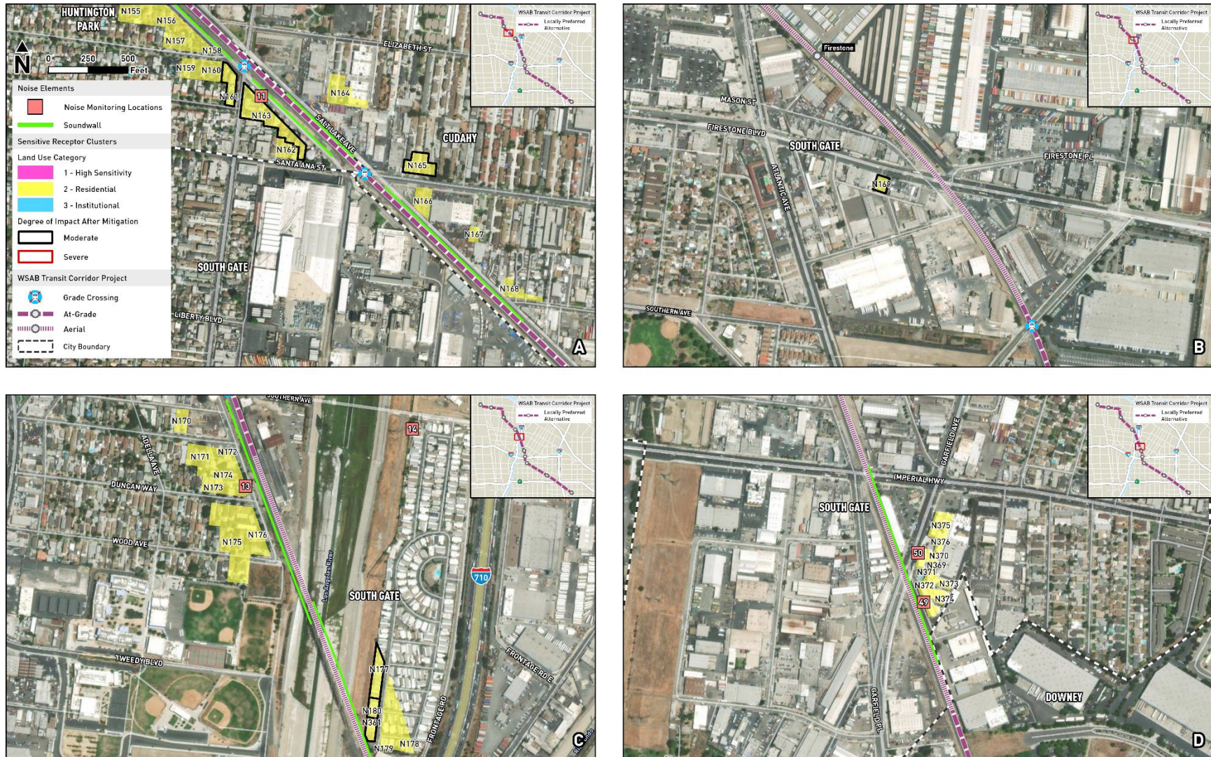
Figure 4.7-7. LRT Noise Impacts Remaining After Mitigation, including Soundwalls (City of Cudahy to City of South Gate)
