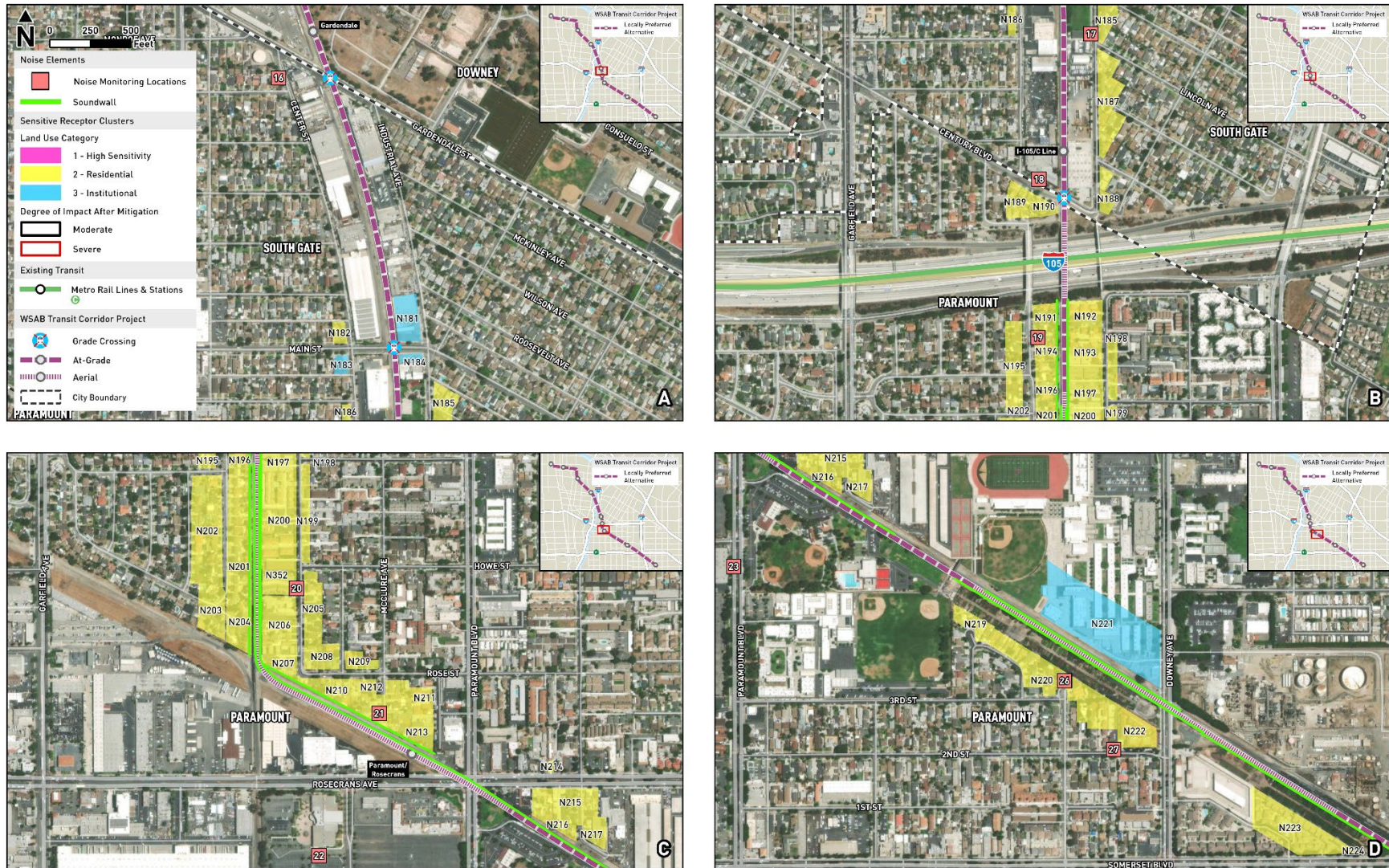
Figure 4.7-8. LRT Noise Impacts Remaining After Mitigation, including Soundwalls (City of South Gate to City of Paramount)
