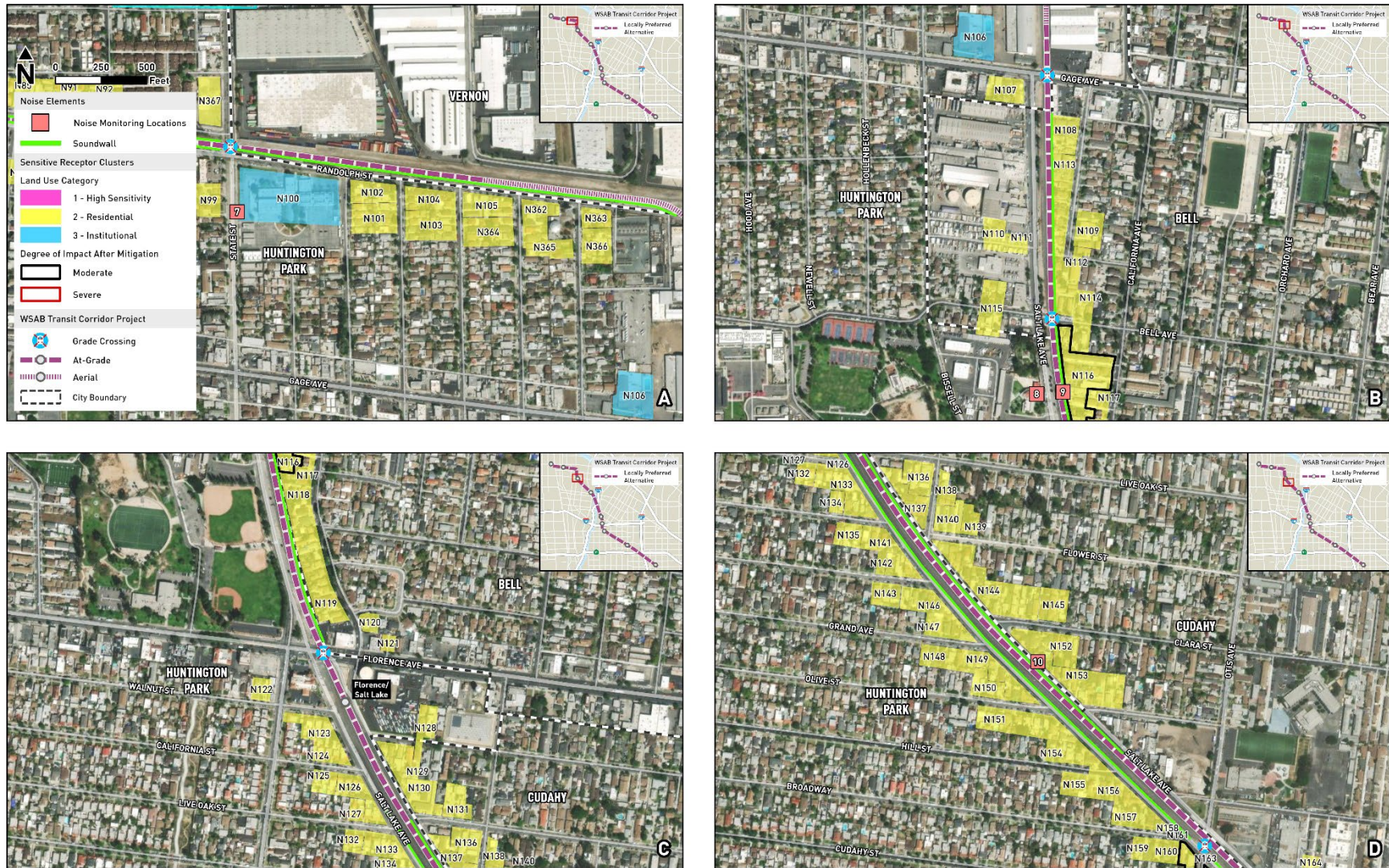
Figure 4.7-6. LRT Noise Impacts Remaining After Mitigation, including Soundwalls (City of Huntington Park to City of Cudahy)
