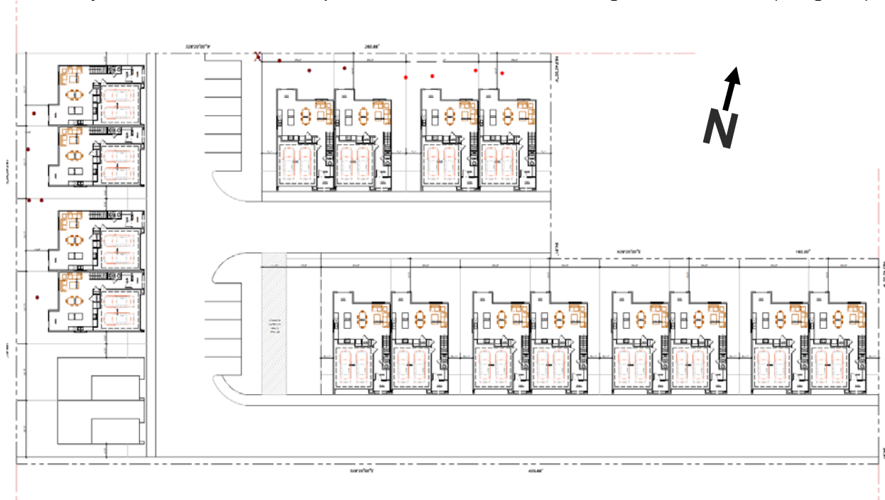
Image #8 – Conceptual site plan. Trees that may be retained (12 total), are shown as brown or red dots. An enlarged site plan can be found in Appendix E of this report.
