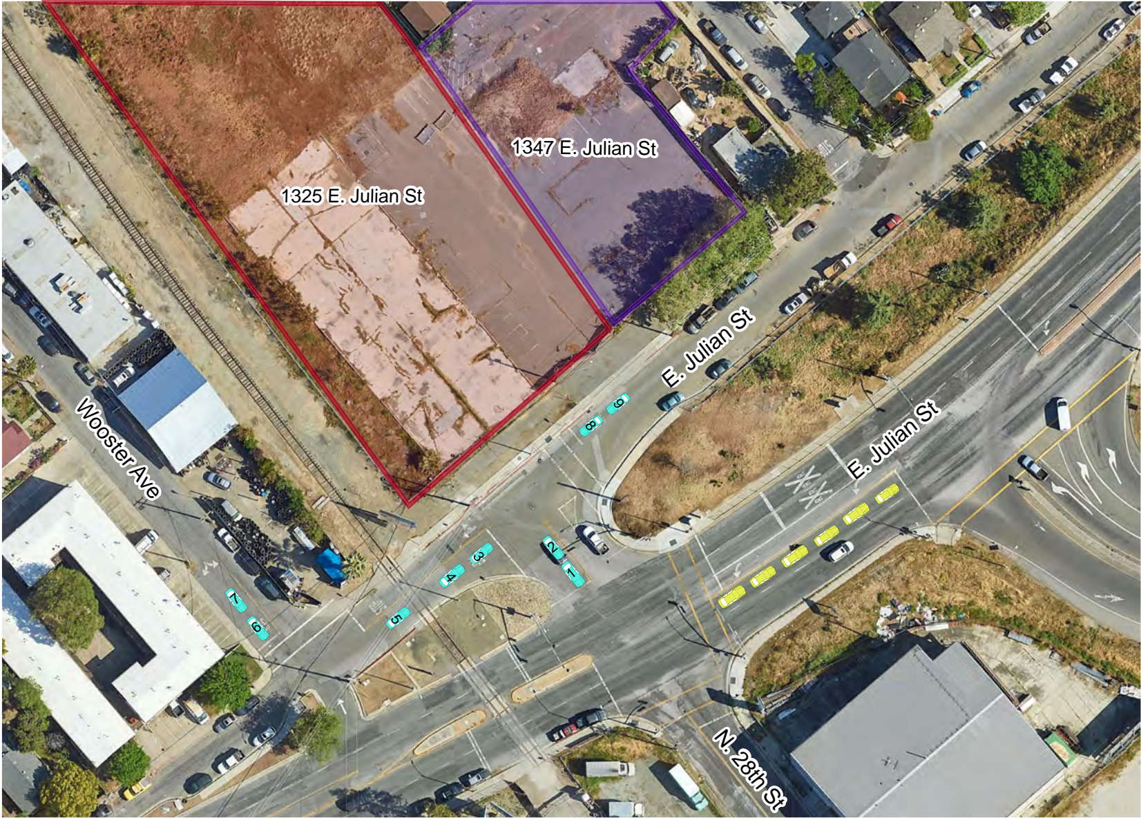
Figure 19 Maximum Observed AM Peak Hour Vehicle Queue at the N. 28th Street/E. Julian Street Intersection
