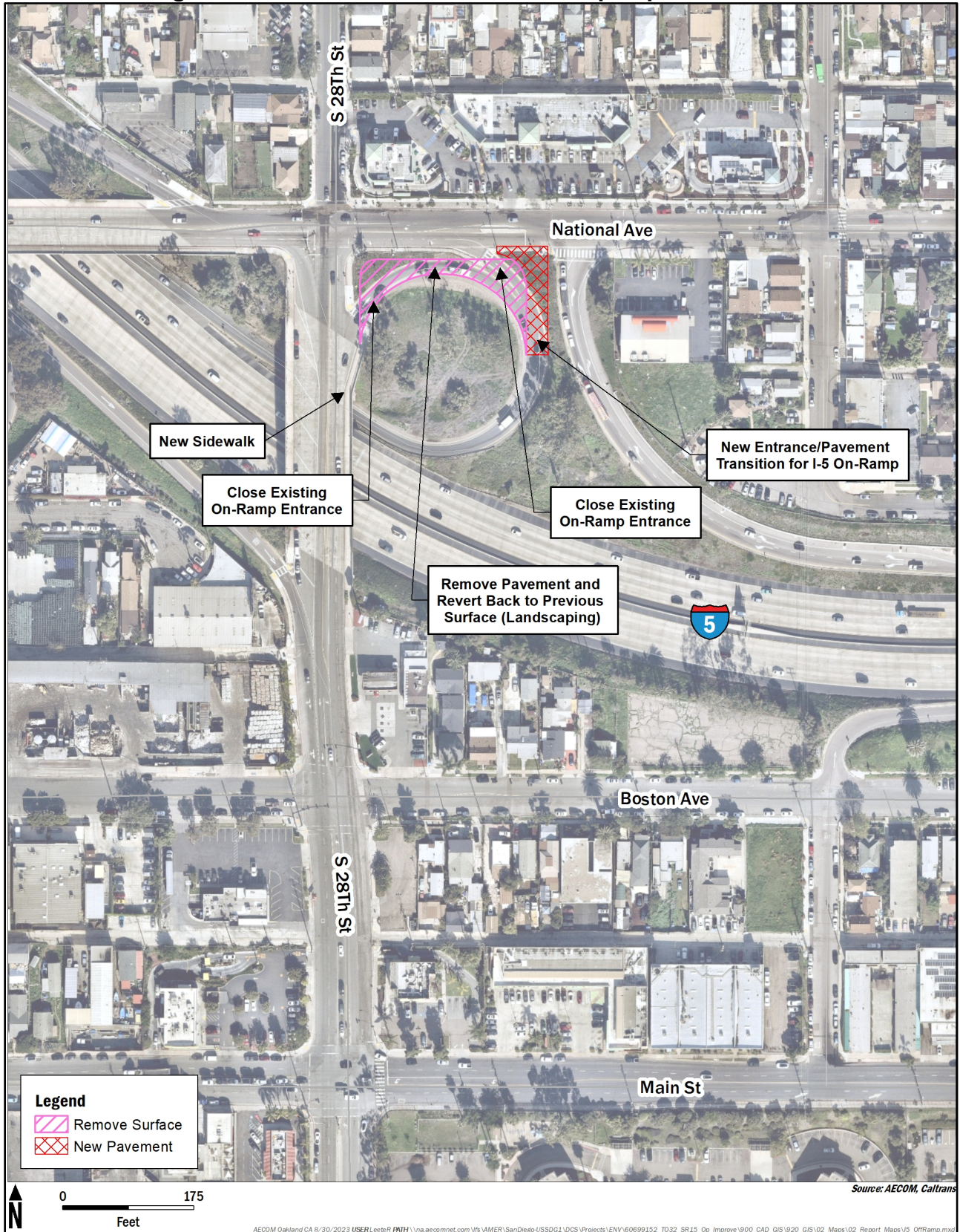
Figure 1-6: I-5/National Avenue On-Ramp Improvements
