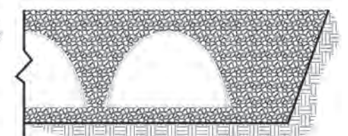
Perimeter Fully Backfilled
