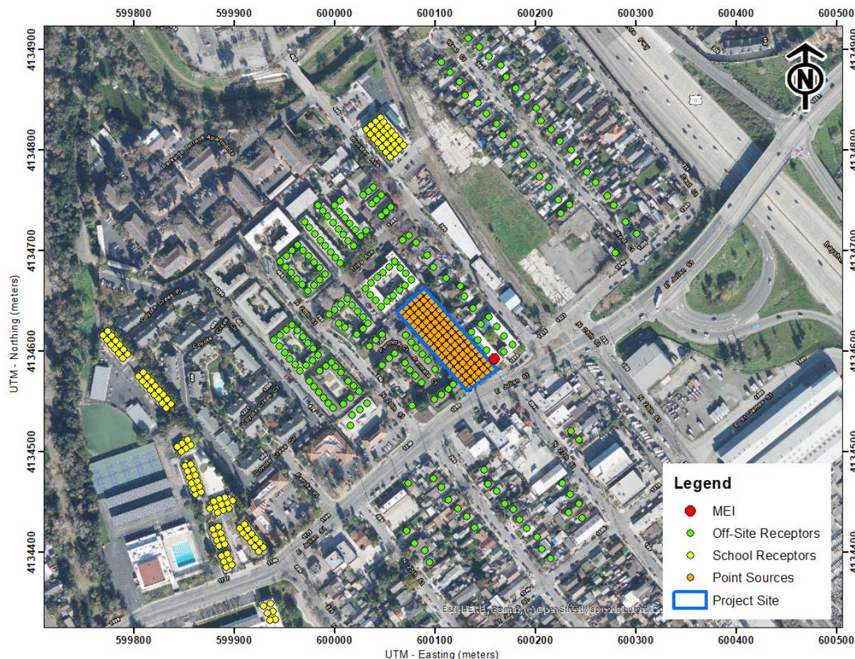
Figure 1. Locations of Project Construction Site, Off-Site Sensitive Receptors, and Maximum TAC Impact (MEI)
