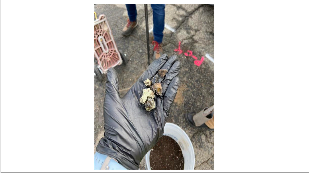
Photograph 1: Spongy material (SM) and red sand core (RSC).
