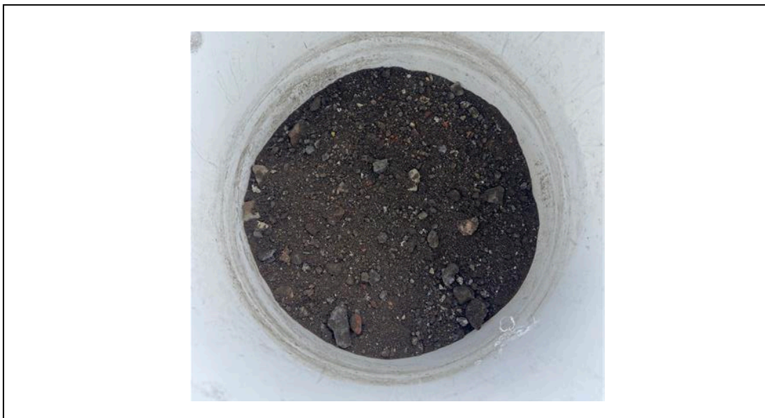
Photograph 2: Example of the dark brown foundry sand (FS).
