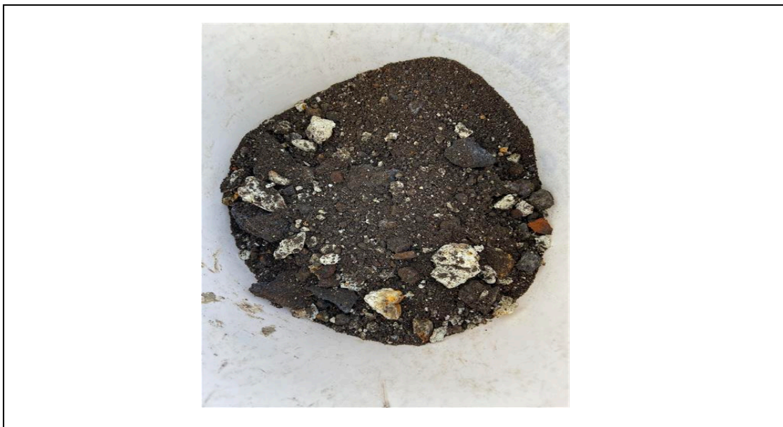
Photograph 6: View of foundry sand from S-31 location.
