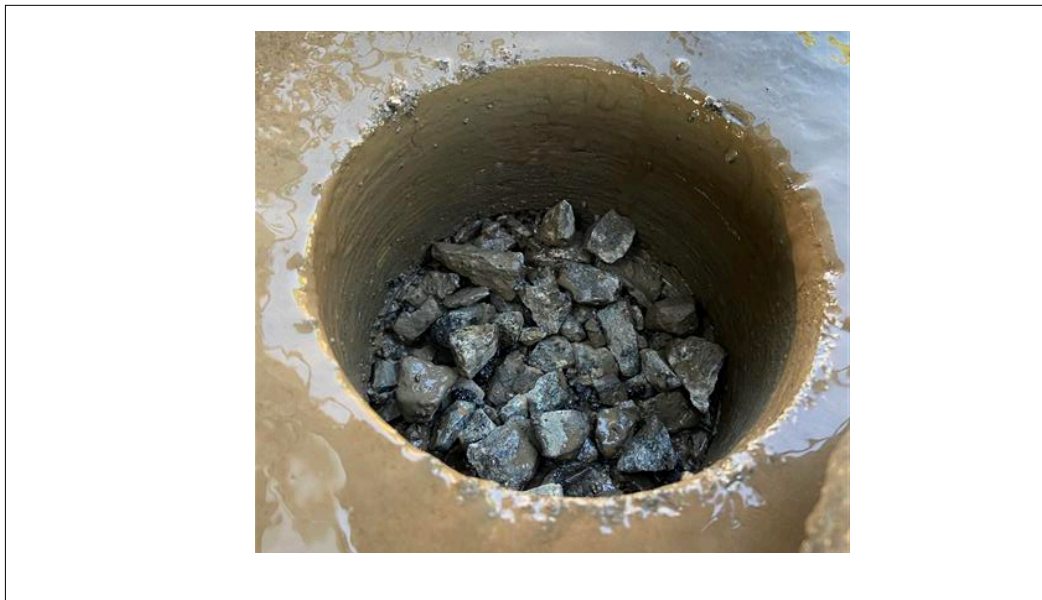
Photograph 4: Base material found underneath the asphalt at sample location S-19. .
