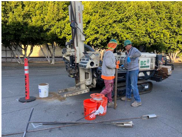
Photograph 11: View of BC2 crew setting up the Geoprobe direct push rig to collect samples
