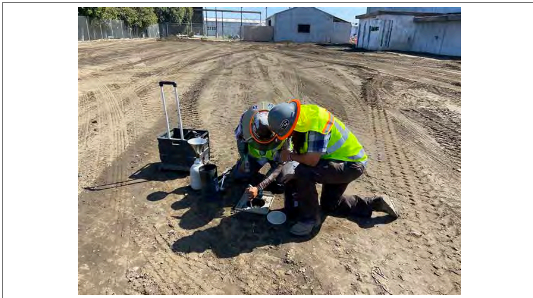
View of GPI conducting geotechnical testing/sampling of compaction (9/3/21).
