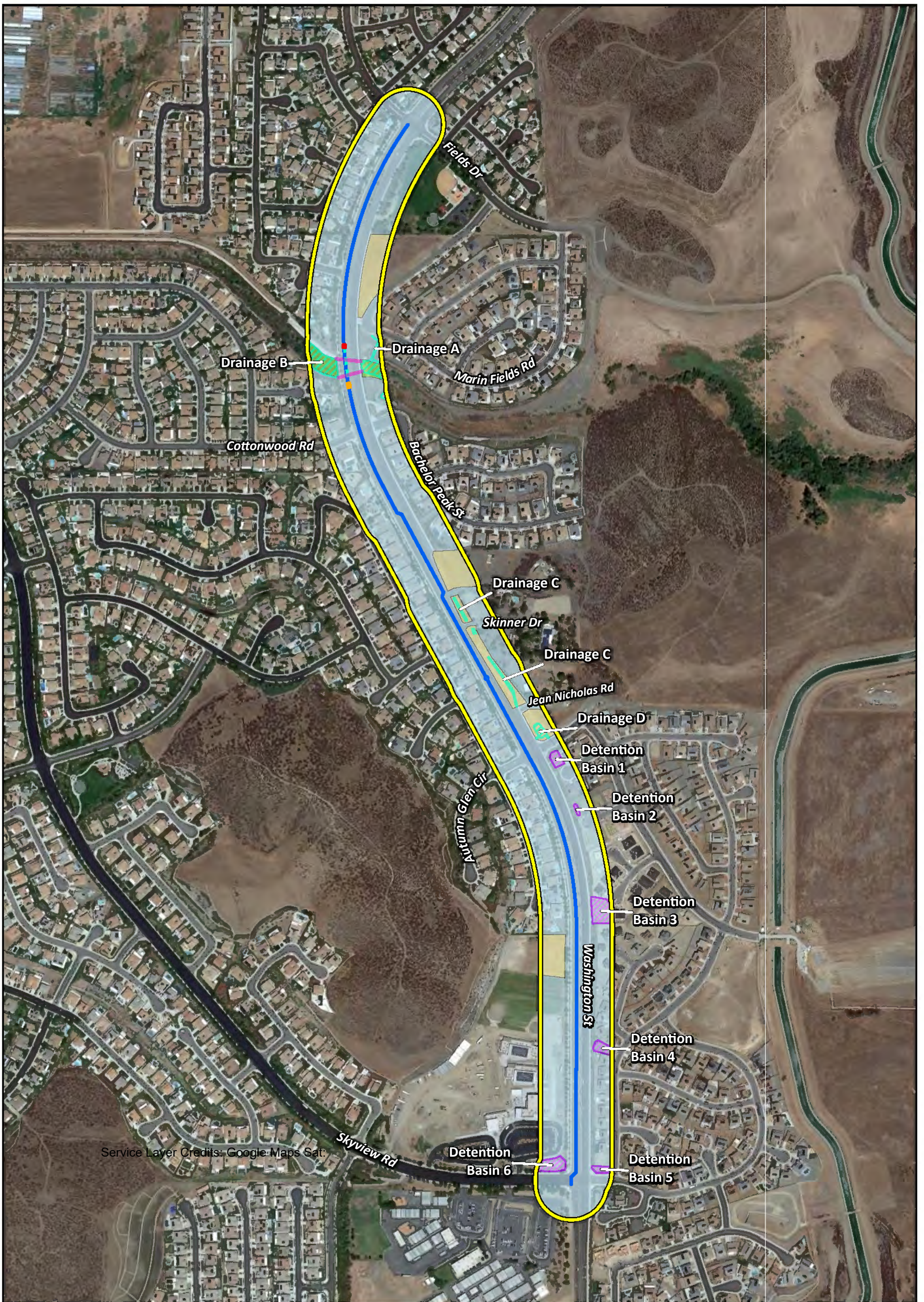
LSA Service Layer Credits: Google Maps Sat 0 250 500 FEET SOURCE: Google (2020) J:\EWD2101.03\GIS\Pro\Washington Street Pipeline Project\Washington Street Pipeline Project.aprx (10/9/2023) Proposed Plans 200-ft Buffer Proposed Project Water Line Jack and Bore Line Jacking Pit Location Receiving Pit Location Vegetation and Land Use Developed/Disturbed (56.07 acres) Nonnative Grassland (4.06 acres) Riparian Scrub (0.66 acres) Potential Jurisdictional Features Drainage Detention Basin Drainage B flow under Washington Street FIGURE 5.4-1 Washington Street Transmission Main Project Vegetation, Land Use, and Potential Jurisdictional Features
