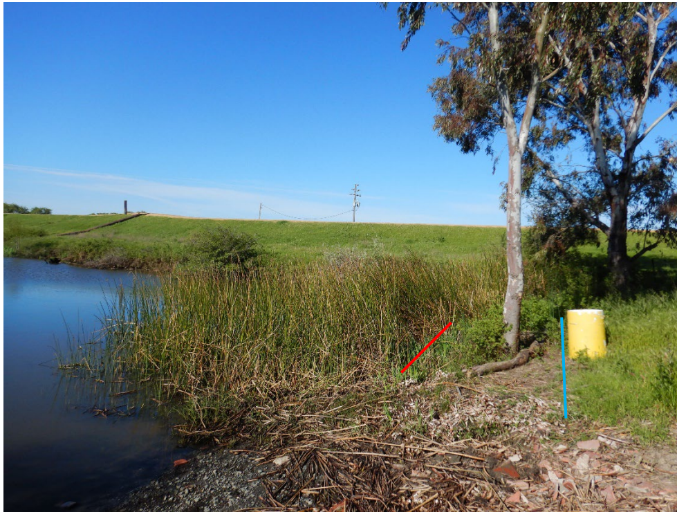
Photo E-1. Transect 1 at MHW (red) and HTL (blue) on Lindsey Slough facing west. HTL indicators include change in vegetation type and presence of organic litter. MHW indicators include change in vegetation type and break in slope.
