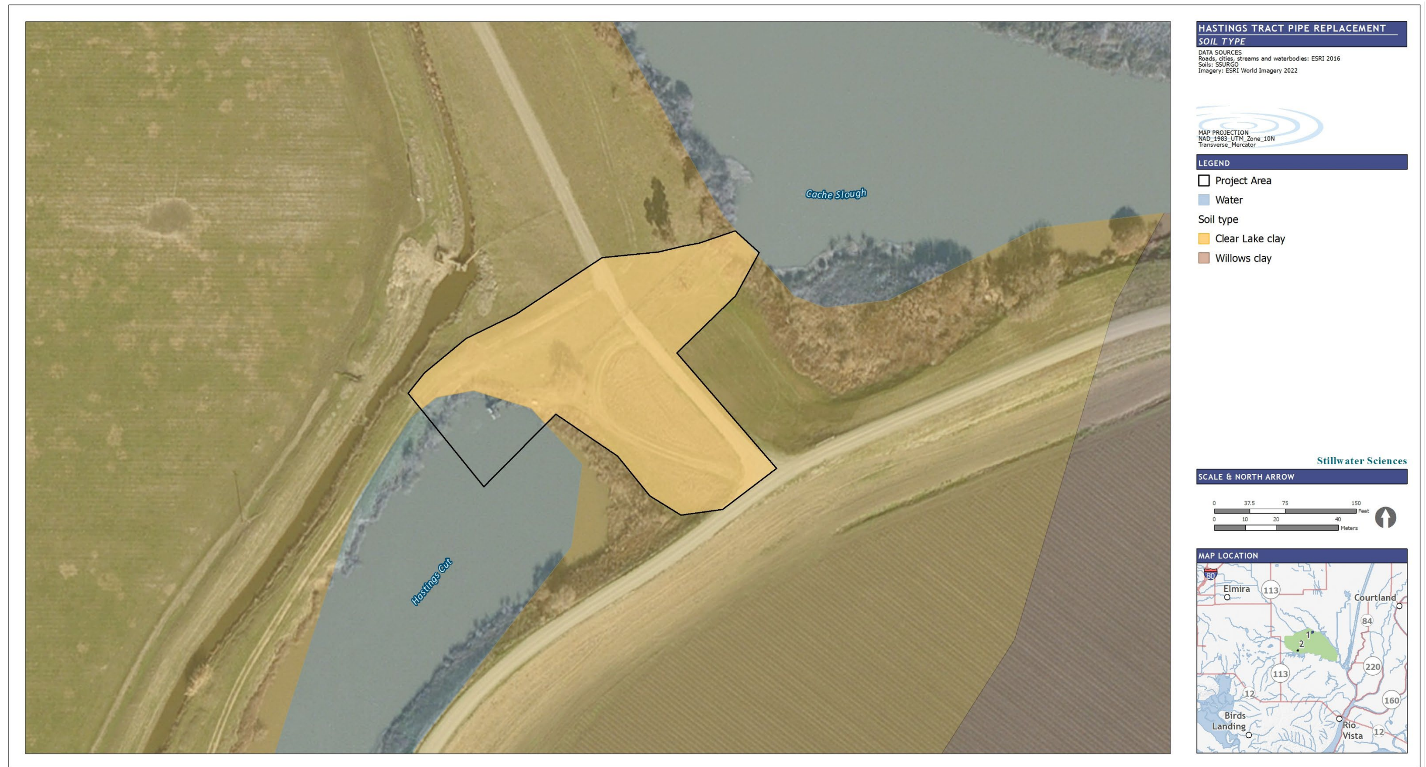
Figure 4a. Soil units in the Hastings Tract Pipe Replacement Project Area, page 1 of 2.
