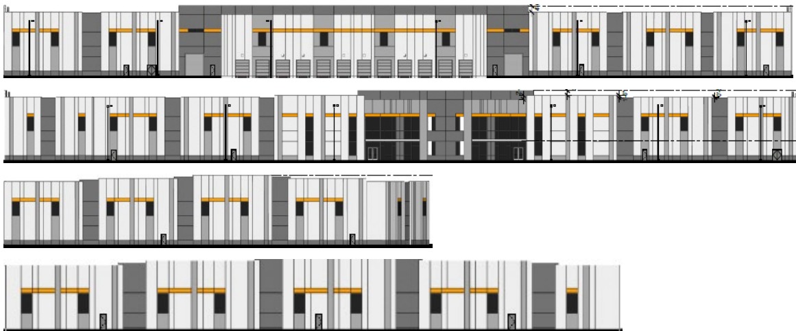
Figure 9. Proposed Facades. The north (top), south (second from top), east (second from bottom), and west (bottom) elevations of the proposed building. The extent of glazing on each façade is shaded in black.
