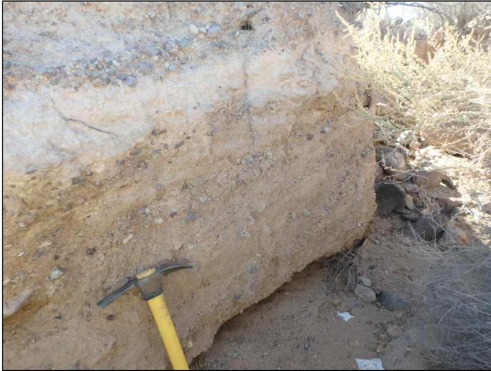
Figure 9. Quaternary older fan deposits (Qof), consisting of tannish-pink, very fine-grained sand and silt, with pebble- to cobble-sized igneous rock clasts, moderately sorted, and exhibiting planar bedding of coarse-grained materials, with more massive layers of fine-grained sediments. View southwest.
