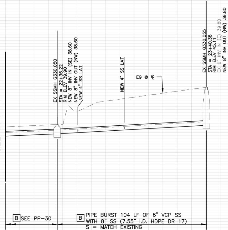
[B] SEE PP-30                      [B] PIPE BURST 104 LF OF 6" VCP SS WITH 8" SS (7.55" I.D. HDPE DR 17) S = MATCH EXISTING
