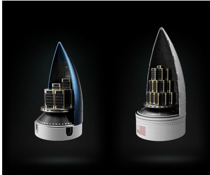
Figure 2-8: Daytona-E Fairing (left) and Laguna-E Fairing (right)
