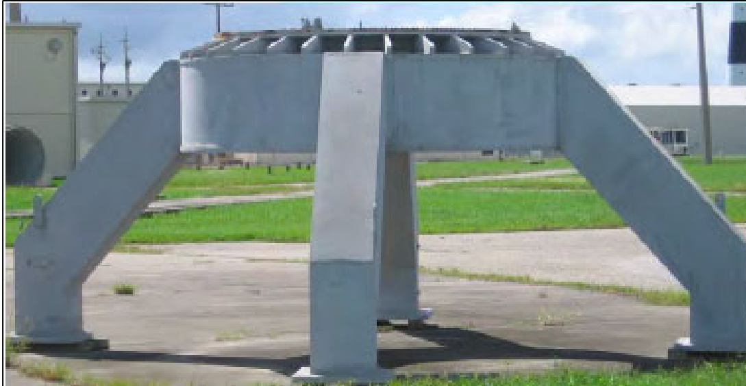
Figure 2-4. Launch stool (conceptual design).
