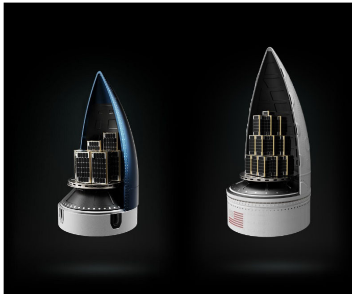
Figure E-3: Daytona-E Fairing (left) and Laguna-E Fairing (right)
