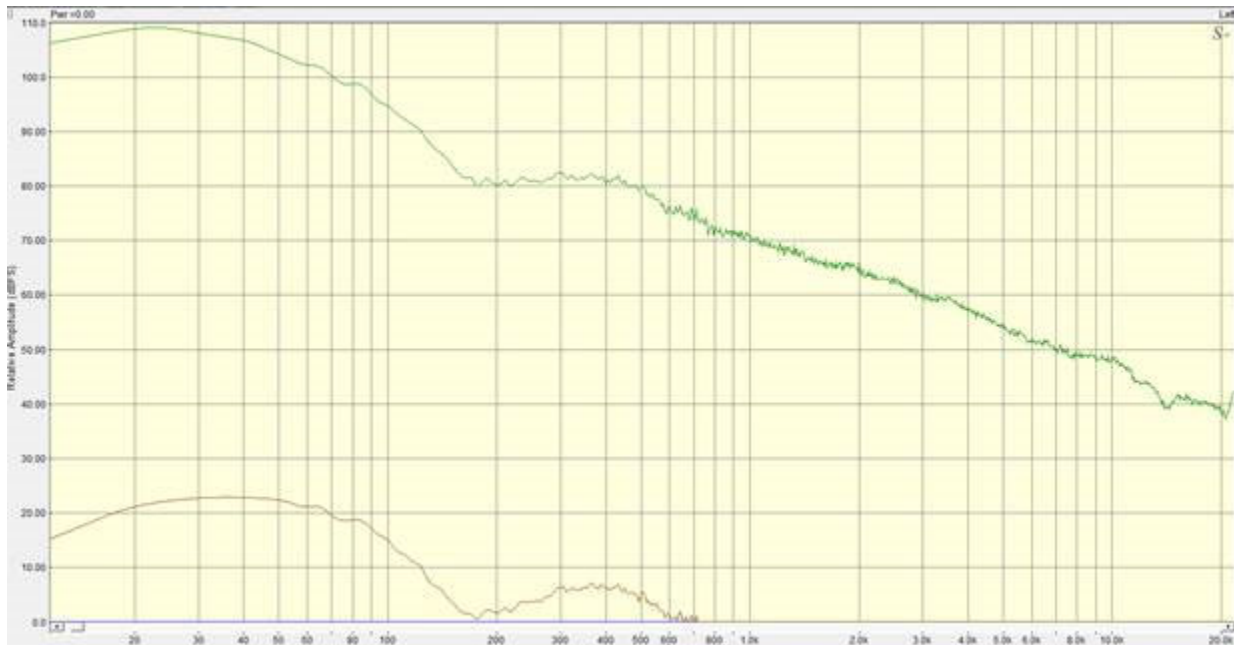
9 10 Figure I-3: Launch peak noise level comparison of unweighted (green) versus Ranidae-weighted 11 (brown) decibels (note: time waveform recording from the Falcon 9 SARah-1 launch)
