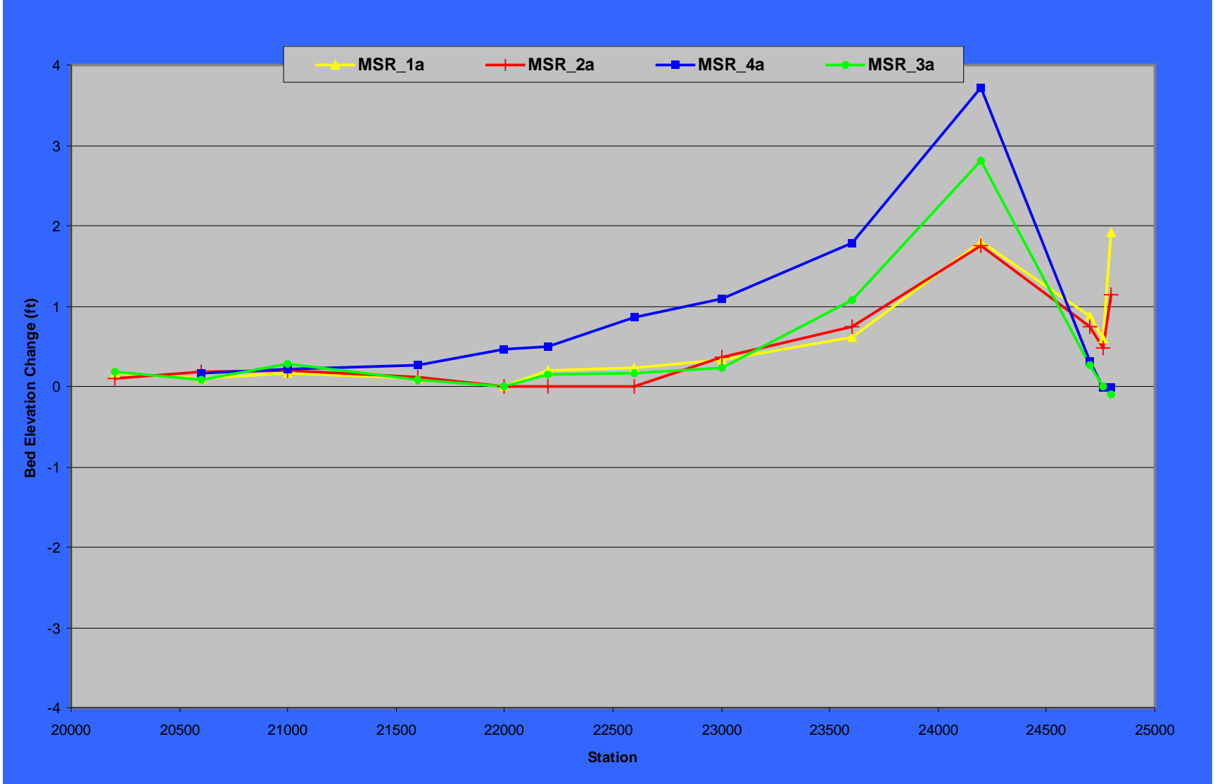
Figure A-16. Bed Elevation Change from Time t=0 to t=1.43 Days for Segment 5, Model Results MSR_1a to 4a.
