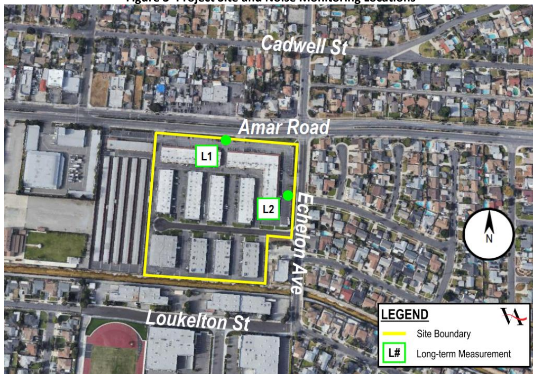
Figure 3—Project Site and Noise Monitoring Locations
