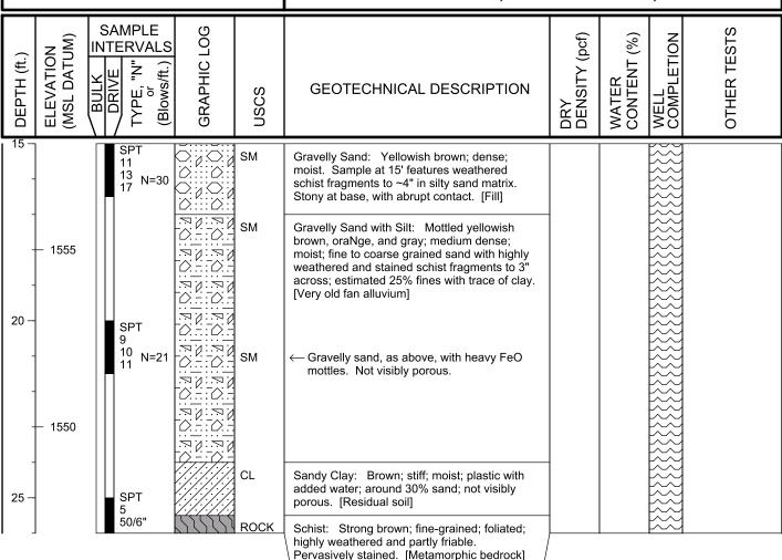
Bottom of boring at 26.0 feet. No groundwater encountered. Boring backfilled with compacted soil cuttings and rapid-set grout.
