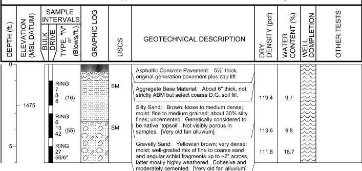
Bottom of boring at 6.0 feet. No groundwater encountered. Boring backfilled with compacted soil cuttings and rapid-set grout.
