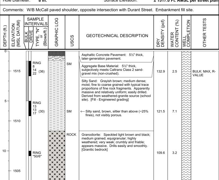
Abrupt refusal encountered at 13.0 feet. No groundwater encountered. Boring backfilled with compacted soil cuttings and rapid-set grout.
