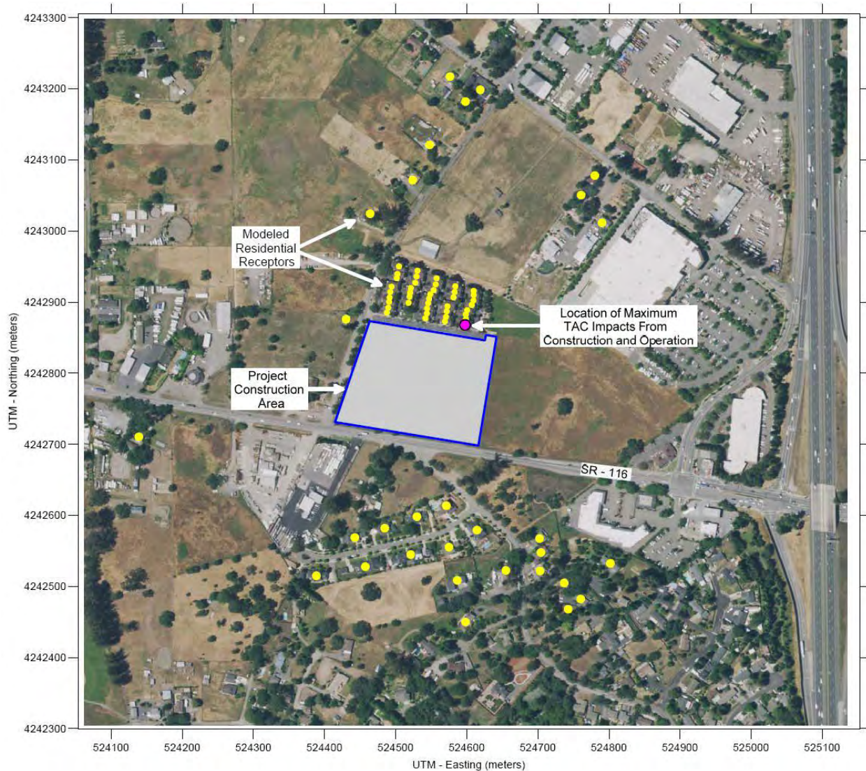
Figure 5.3.1 Location of Project Construction Site, Off-site Sensitive Receptors, and Maximum TAC Impact (MEI)
