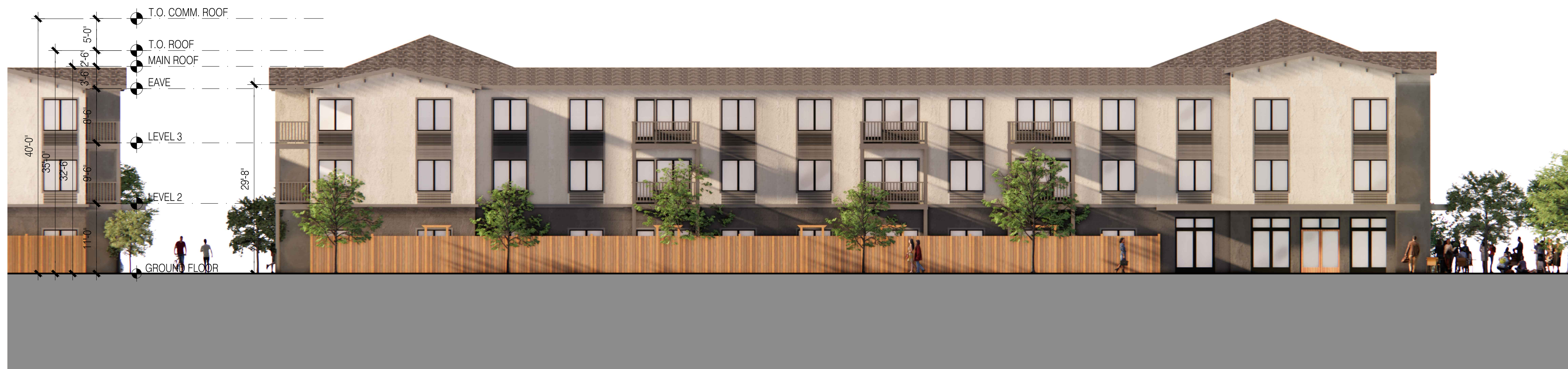
4 BUILDING A - NORTH ELEVATION 3/64" = 1'-0" @ 11X17 3/32" = 1'-0" @ 24X36
