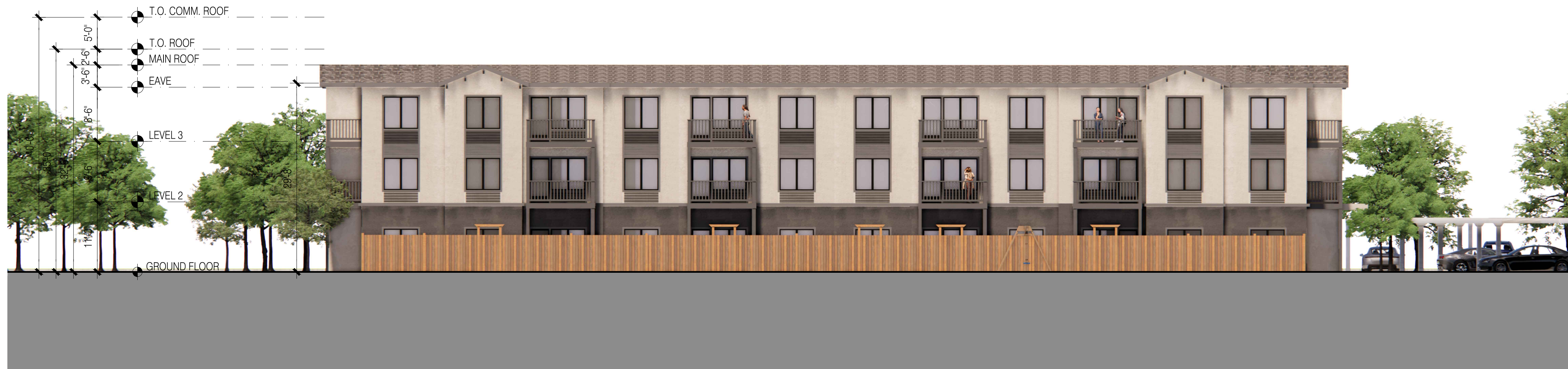
4 BUILDING F - EAST ELEVATION 3/64"=1'-0" @ 11X17 3/32" = 1'-0" @ 24X36
