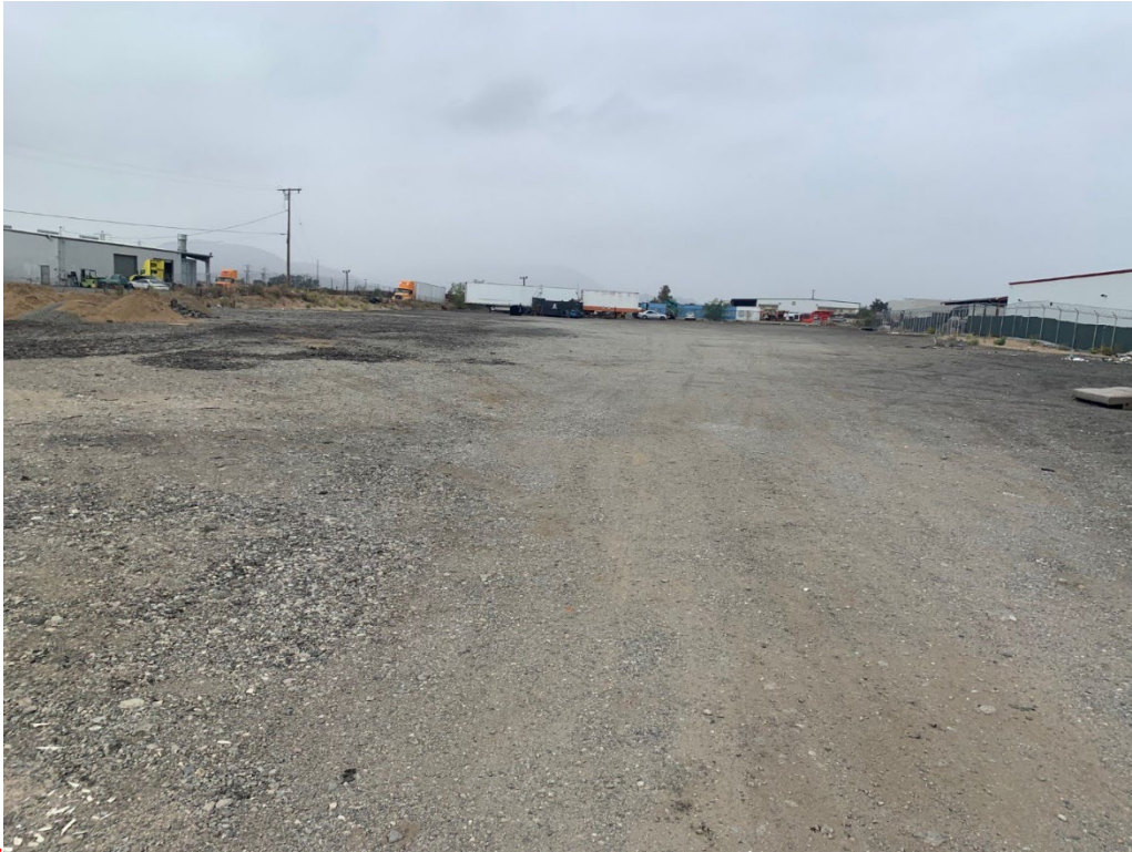
Photograph 1. Looking west from the eastern boundary. The site is paved or covered with gravel. Open Delhi Sands occur at the base of the perimeter fence lines around the site. Sands are moderately to heavily impacted by truck storage, contaminated with industrial waste, and mixed with gravel.
