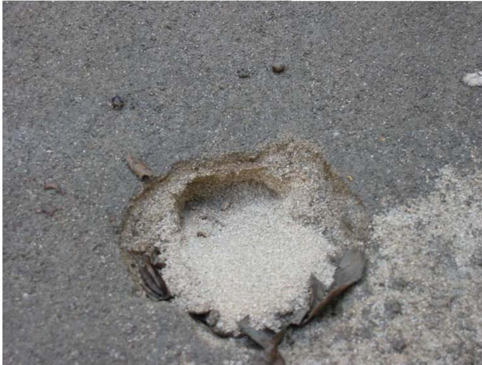
Figure 7 Formation of Clogging Crust on Filter Bed
