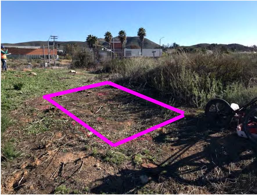
Pink outline shows location of possible UST. Thick vegetation prevented GPR from scanning additional area.
