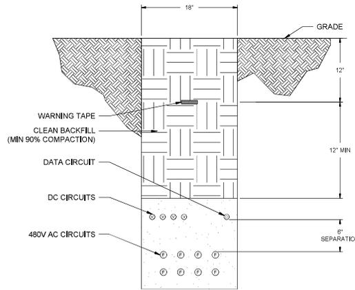
1 AC FEEDER TRENCH WITH DC SOURCE CIRCUIT & DATA
