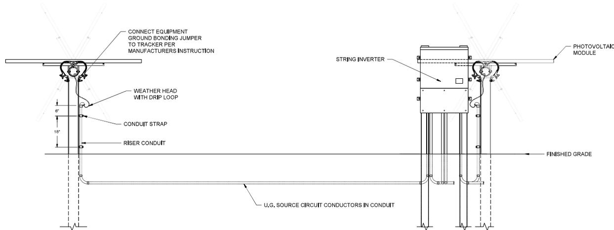
4 DC SOURCE CIRCUIT (JUMPER) TRENCH DETAIL
