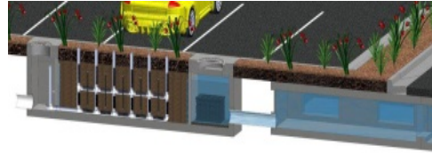
Horizontal Flow Biofiltration System
