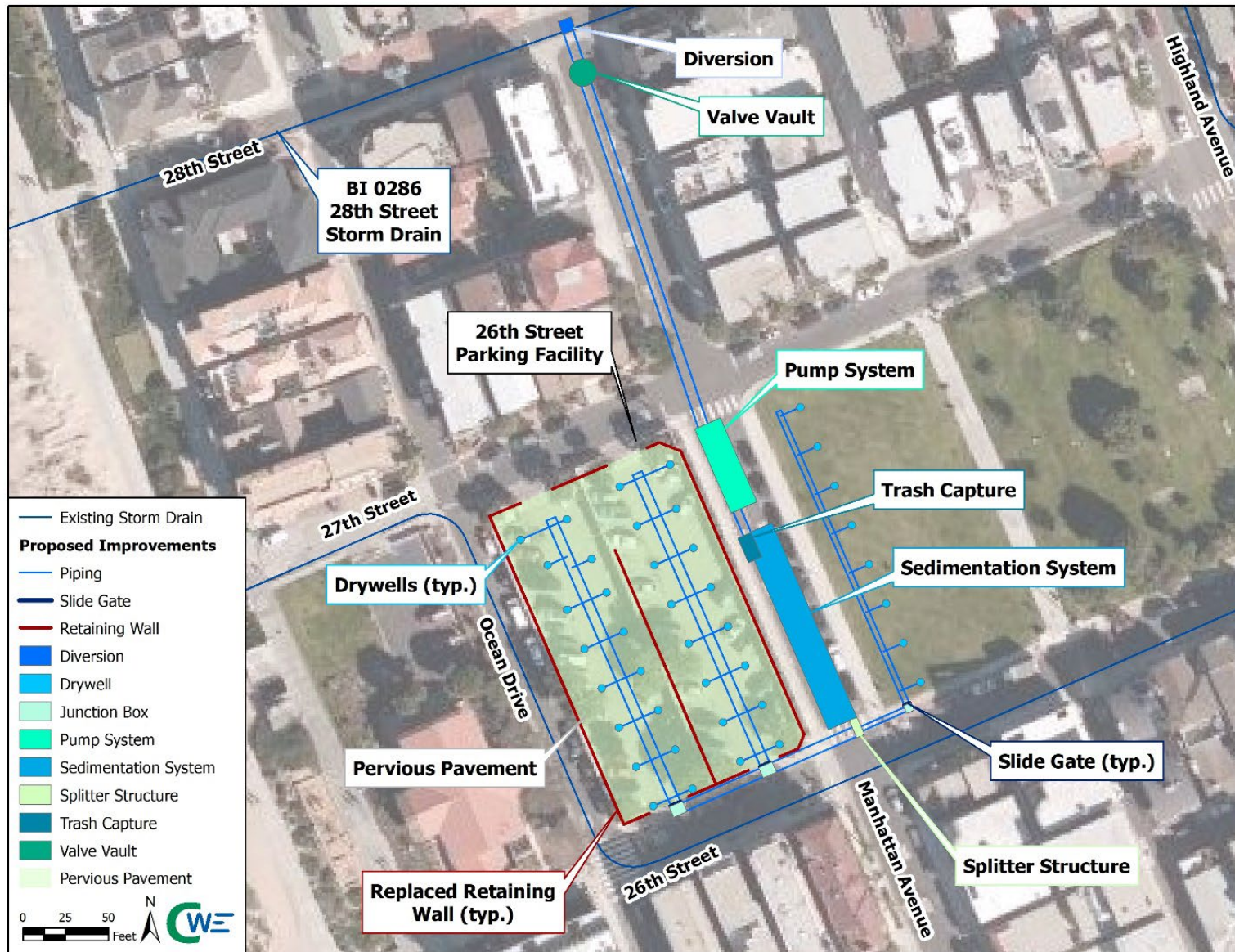
Figure 1-3 Stormwater Infiltration Concept
