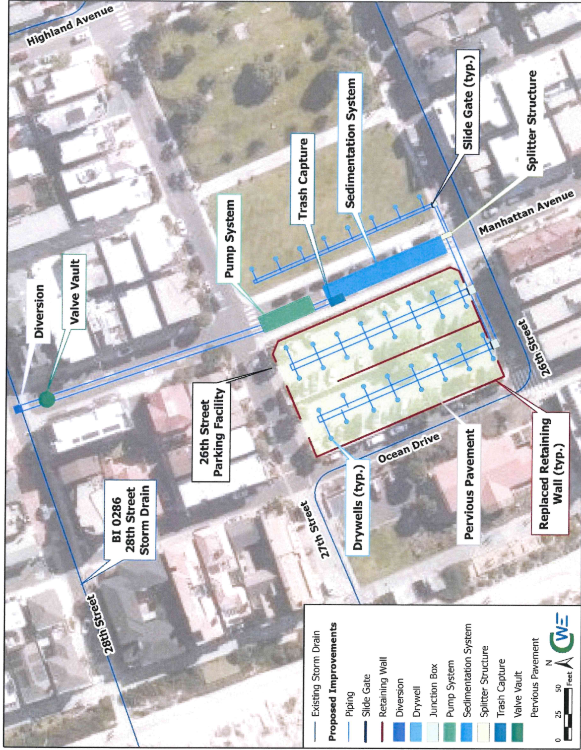
Figure 2 Stormwater Infiltration Concept
