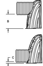
CUSTOM PRECORED INVERTS ARE AVAILABLE UPON REQUEST. INVENTORIED MANIFOLDS INCLUDE 12-24" (300-600 mm) SIZE ON SIZE AND 15-48" (375-1200 mm) ECCENTRIC MANIFOLDS. CUSTOM INVERT LOCATIONS ON THE MC-3500 END CAP CUT IN THE FIELD ARE NOT RECOMMENDED FOR PIPE SIZES GREATER THAN 10" (250 mm). THE INVERT LOCATION IN COLUMN 'B' ARE THE HIGHEST POSSIBLE FOR THE PIPE SIZE.
