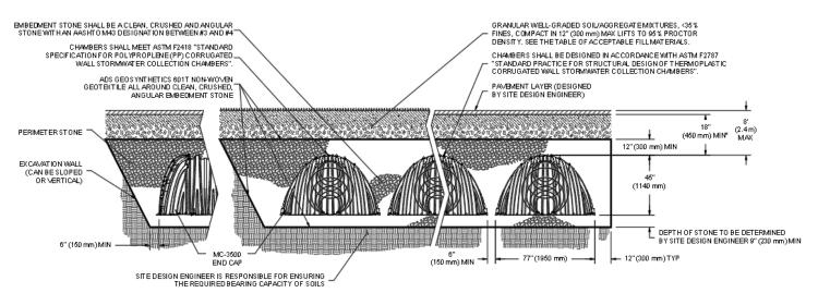
MINIMUM COVER TO BOTTOM OF FLEXIBLE PAVEMENT. FOR UNPAVED INSTALLATIONS WHERE RUTTING FROM VEHICLES MAY OCCUR, INCREASE COVER TO 24"
