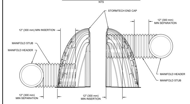
NOTE: MANIFOLD STUB MUST BE LAID HORIZONTAL FOR A PROPER FIT IN END CAP OPENING.
