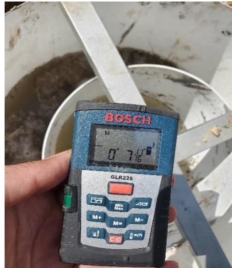
Figure 23: Accuracy of Reading water level by laser meter. Test was done by reading level of the water at specific time intervals
