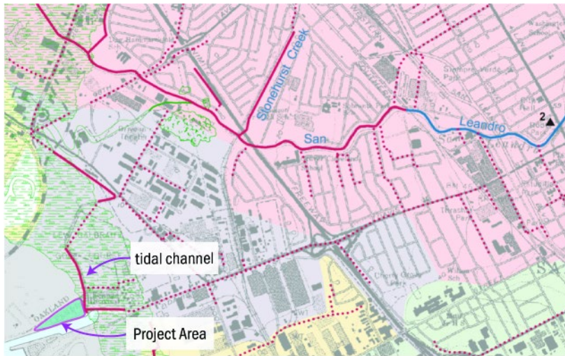
Figure 3-1. Detail view of the Creek and Watershed Map of Hayward and San Leandro , showing the Project location and the tidal channel in question. The engineered channel (solid red line) is connected to underground culverts and storm drains (dashed lines) without connectivity to a stream or river, including San Leandro Creek.
