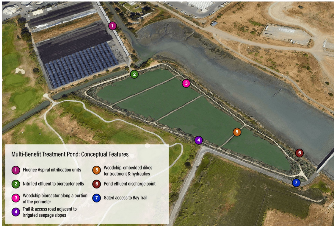
Figure 2.9. Southeast-facing aerial view of anticipated conditions following implementation of the Proposed Project
