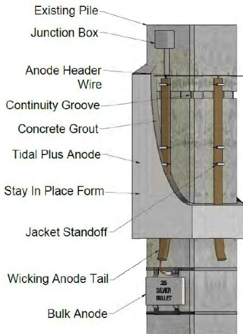
Figure G-1. Galvanic Anode Jacket System
