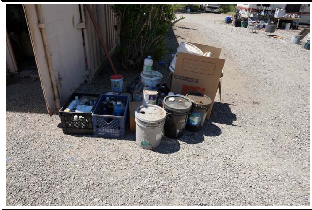
Photograph Number 15: View of numerous pails and containers of hydraulic oil, lubricants and maintenance chemicals stored adjacent to maintenance shop.
