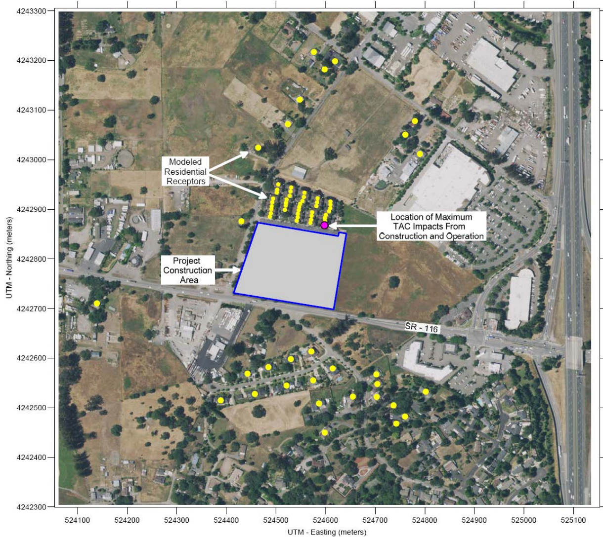
Figure 1. Location of Project Construction Site, Off-Site Sensitive Receptors, and Maximum TAC Impact (MEI)
